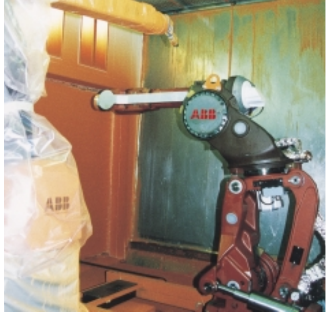
Advanced production technology is used in the manufacture of the new compact robot. Here, an ABB painting robot applies the primer coat to an IRB 6400C.
