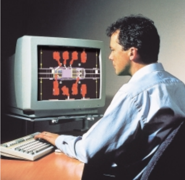
With the help of simulation software, spot welding station configurations can be optimized before the equipment is installed. The spot welding program is generated in off-line mode.
