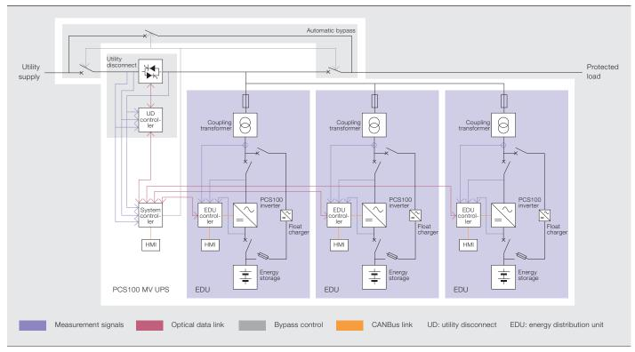
More frequently, the UPS is required to condition the incoming power – removing sags and short-duration phenomena caused by faults in the external power network. Here, ultracapacitor energy storage is used. For such high-power demands, the small footprint of ultracapacitor energy storage – with a power density of 1,000 kW/m<sup>2</sup> a reality – has a clear advantage.
