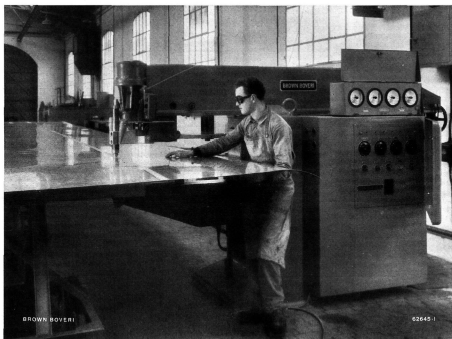
Fig. 83. — Probably the largest spot welder in existence, installed at the workshops of the Swiss Car and Elevator Corporation, Schlieren (Switzerland).
