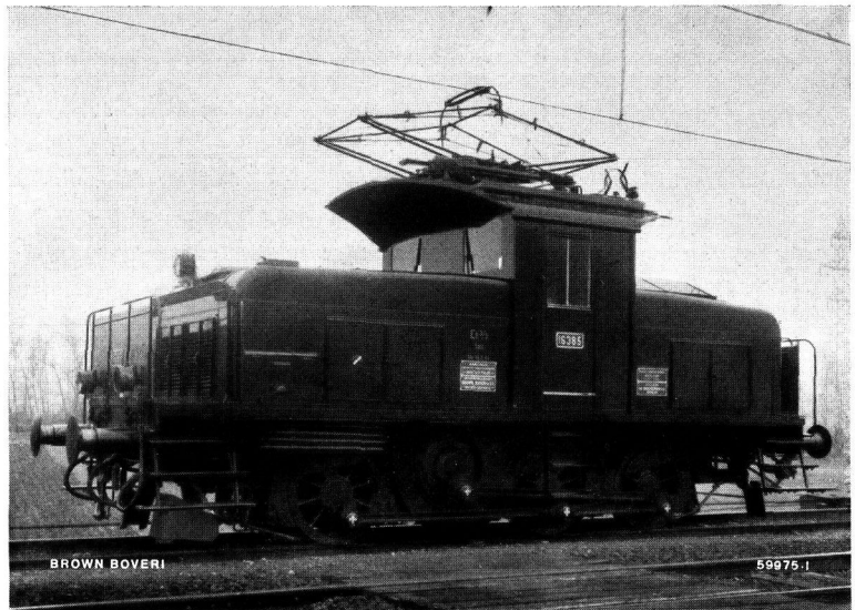
Fig. 115. — Swiss Federal Railways shunting locomotive Ee 3/3.
