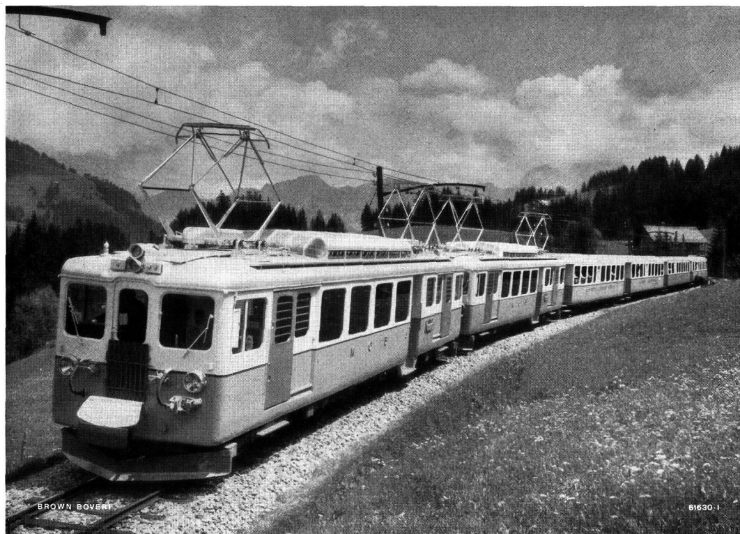
Fig. 121. — Lightweight passenger train on Montreux—Bernier-Oberland Railway, comprising two motor-coaches with multiple-unit control and four new trailing coaches.
