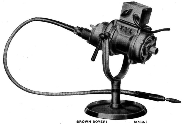
Fig. 54. — 0.55 kW three-phase motor combined with six-stage change-over gearing for the drive of various tools through a flexible shaft. A mobile electric tool for a hundred and one jobs.
