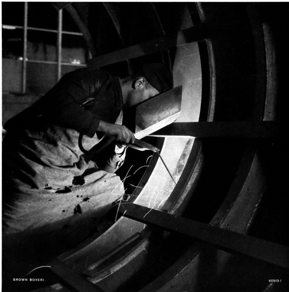
Welding a fabricated motor casing.
