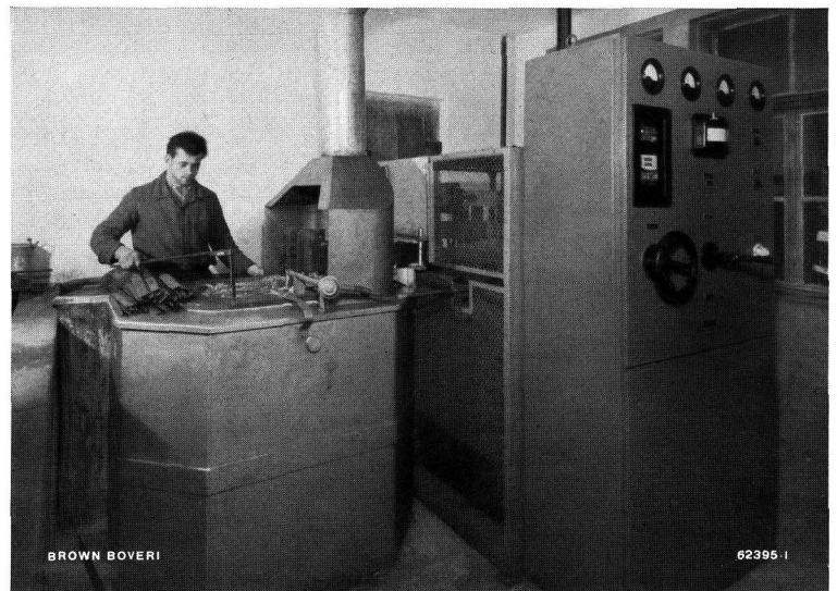
Fig. 81. — Electrode salt-bath furnace plant in service.
