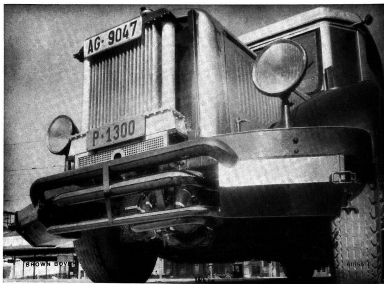
Fig. 110. — Motor bus of the Swiss Telegraph and Telephone Administration with exhaust turbo-chargers for supercharging an Imbert wood gas generator.
