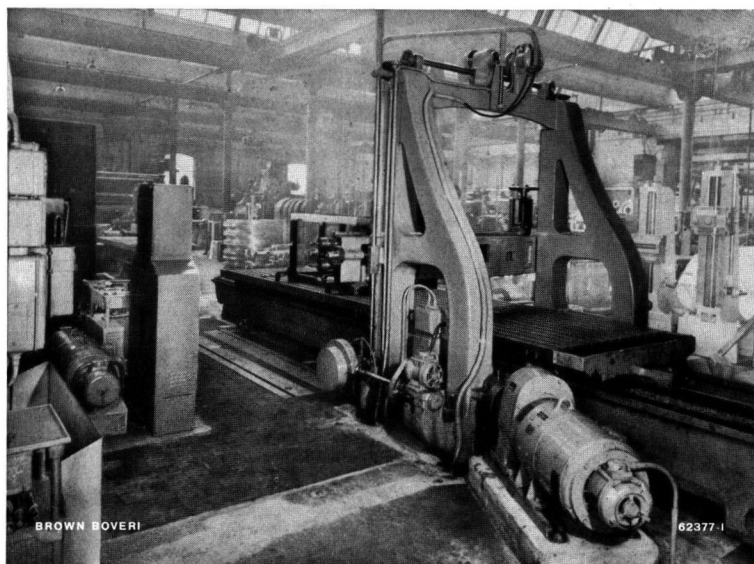
Fig. 76. — Modernized 52-year old double standard planing machine. Brown Boveri rapid reversing planing machine drive and feed and transverse slide displacement drives. Cutting and return speed independent of each other in a ratio of more than 1:10, adjustable without steps, so that this "veteran" now operates like a modern machine. Readily understood and simple operation by means of suspended-type push-button station.
