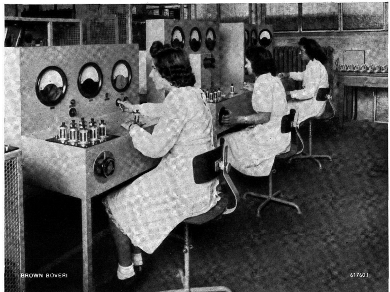
Fig. 134. — Testing tables for the electrical checking of valves.
