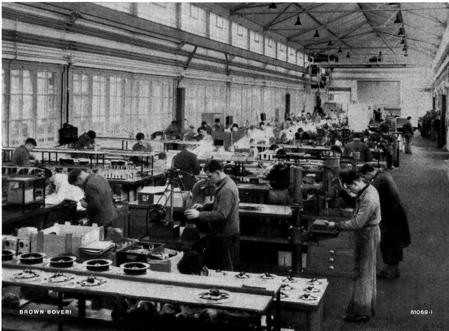
Fig. 127. — Part of a machine and erection shop for transmitters in the Company's factory for high-frequency equipment. The manufacture of such products, which require little material but a large number of working hours, is especially desirable on account of the difficult position of Switzerland with regard to raw materials and in view of her highly skilled workmen.
