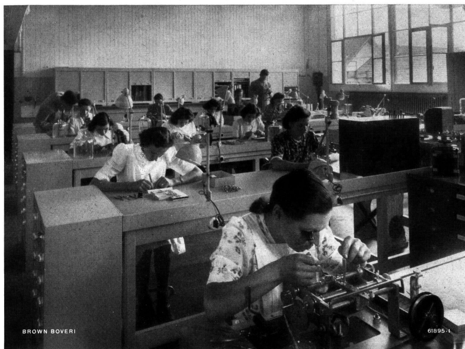
Fig. 128. — Assembly of small and medium-size valves up to 1 kW.
