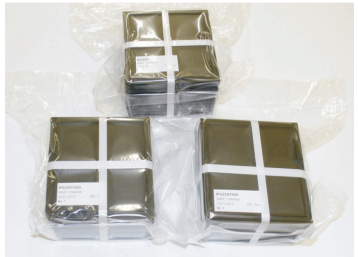
Fig 3: Packing of bare dies in waffle packs
