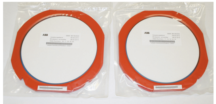
Fig 4: Packing of sawn wafer dies on adhesive tape
