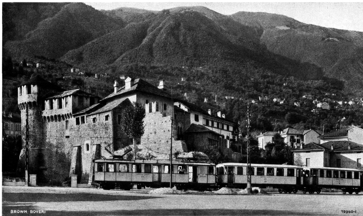
Centovalli Railway; train composed of motor coach and two trailers.
