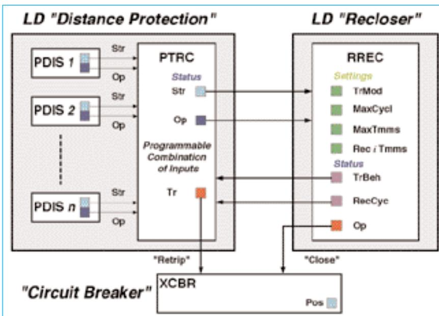
Figure 4: Connection between distance protection and recloser functions
