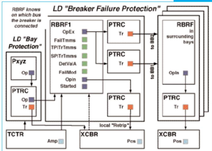
Figure 5: Breaker failure protection in double busbar arrangement
