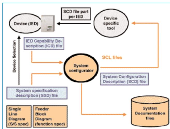
Figure 7: The engineering process using SCL files
