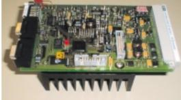
Also, the modem already has a complete communication channel analysis tool that gives the user the opportunity to analyze the suitability of his power system for communication purposes. In future, the modem will achieve a higher degree of automation so that adaptive carrier selection will be possible.
