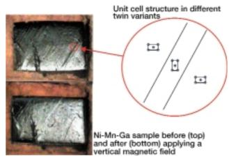
The basic MSM effect mode is extensional strain where the sample shortens in the direction of an applied magnetic field and extends in one of the perpendicular directions. The third dimension remains the same and the total volume of the sample does not change. Reversion of the shape change can be achieved by using a perpendicular magnetic field.
