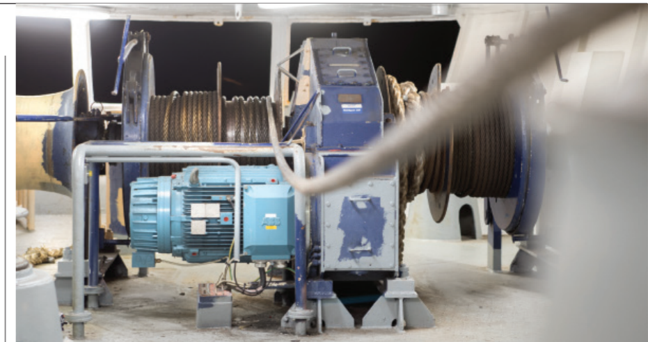
The smaller, lighter SynRM motor was mounted using the existing winch gearbox
