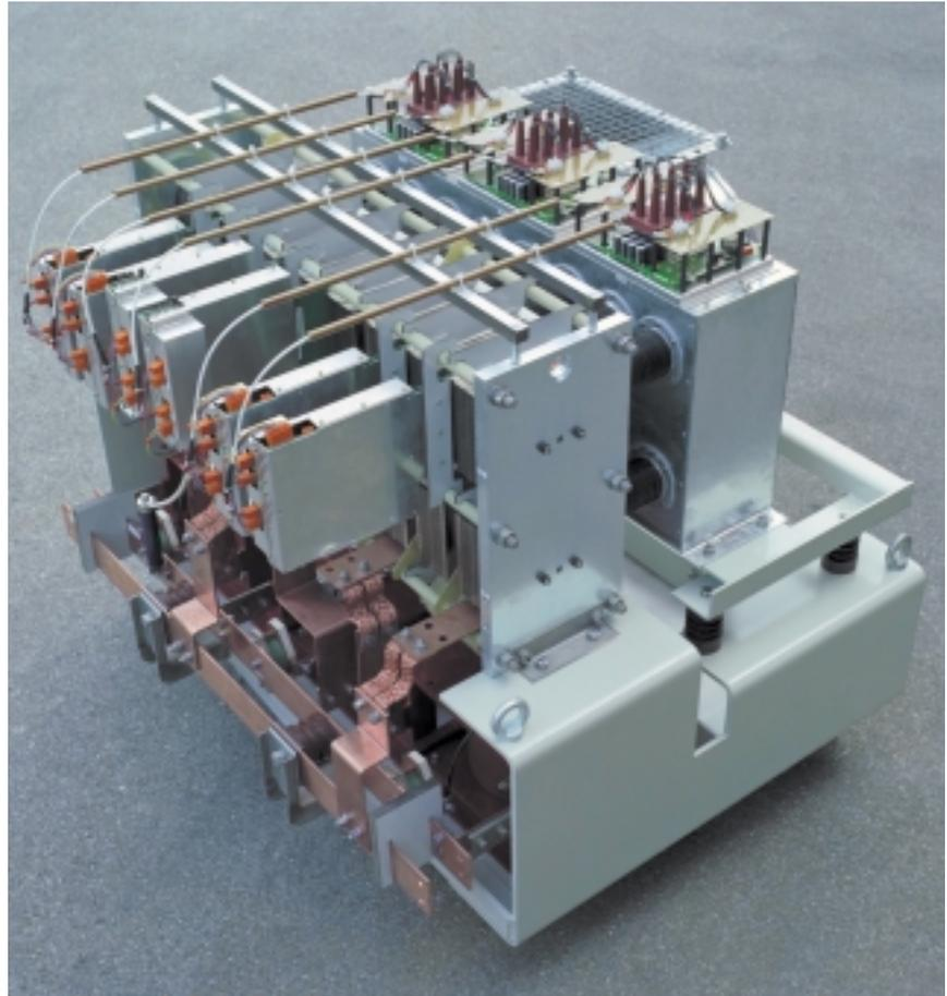
**Three-phase, IGCT-based converter rated at 1.5 MW and 1 kHz, from ABB Industrie AG. The converter is for a dynamic voltage restorer.**
