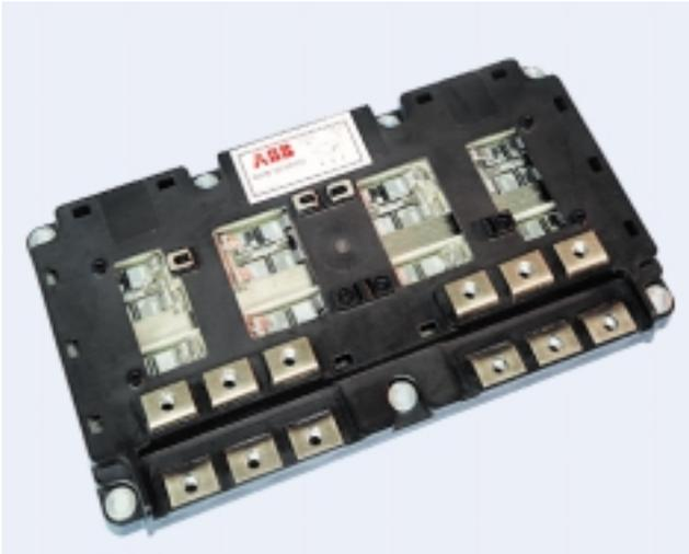
**IGBT module rated 2500 V/1200 A (single switch)**
