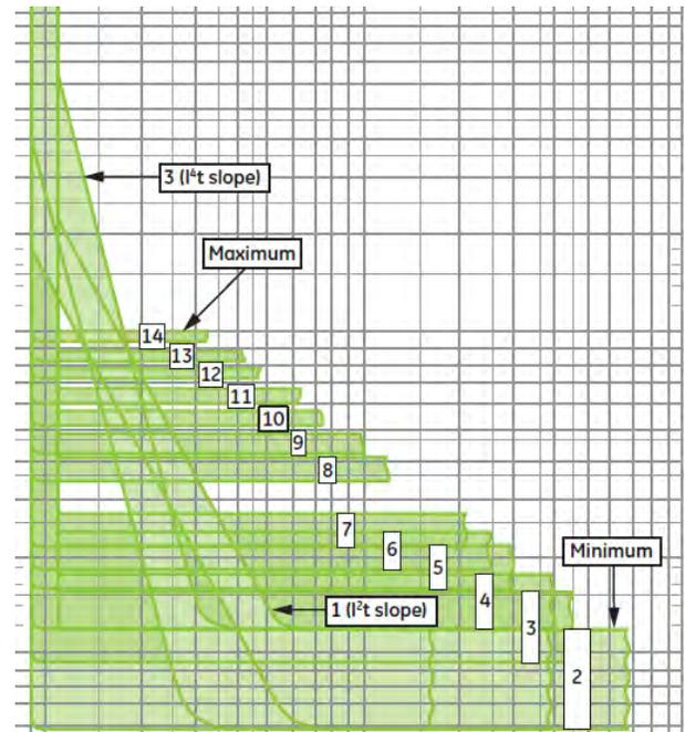
**Figure 6-4: Ground Fault Sum Slope, Option 2**
