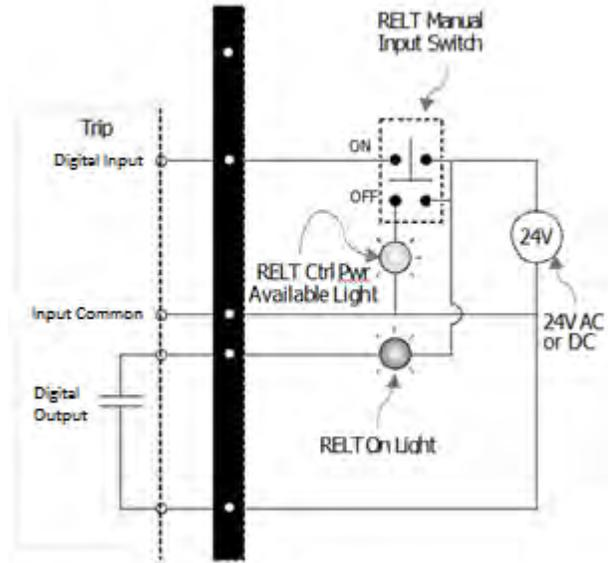
Figure 10-2: RELT Connection without Positive Feedback from EntelliGuard TU Trip Unit
