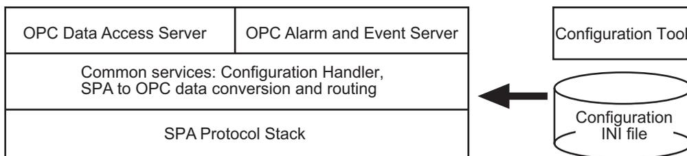
*Figure 3-1: Software component structure of the SPA OPC Server*
