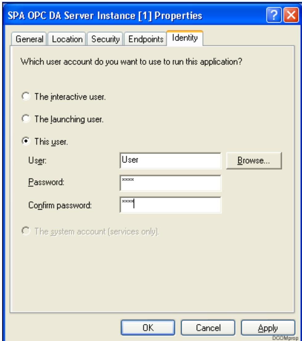
Figure 4-10: Example of DCOM properties
