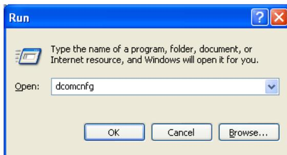
*Figure 4-8: Launching the `dcomcnfg`*
