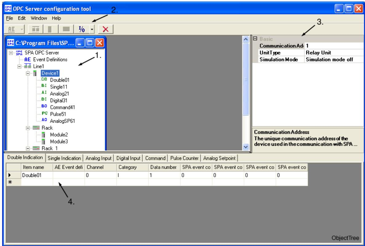
Figure 4-2: Example view of the SPA OPC Server configuration tool
