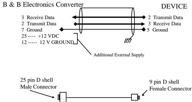
Figure 3 – RS 232 Cable Connections When No Handshaking Is Used. See Figure 1 For Jumper Settings. DTE To DCE Connection. (9 Pin To 25 Pin RS 232 Connection)
