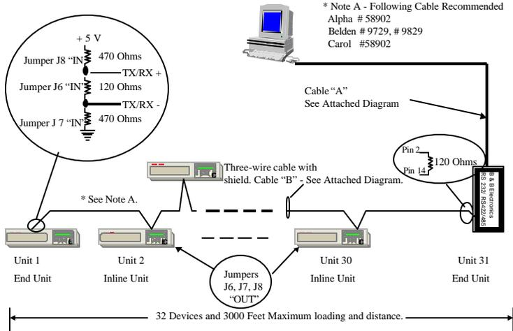
Figure 7 – Termination Using Internal Jumpers And Converter As An End Unit.
