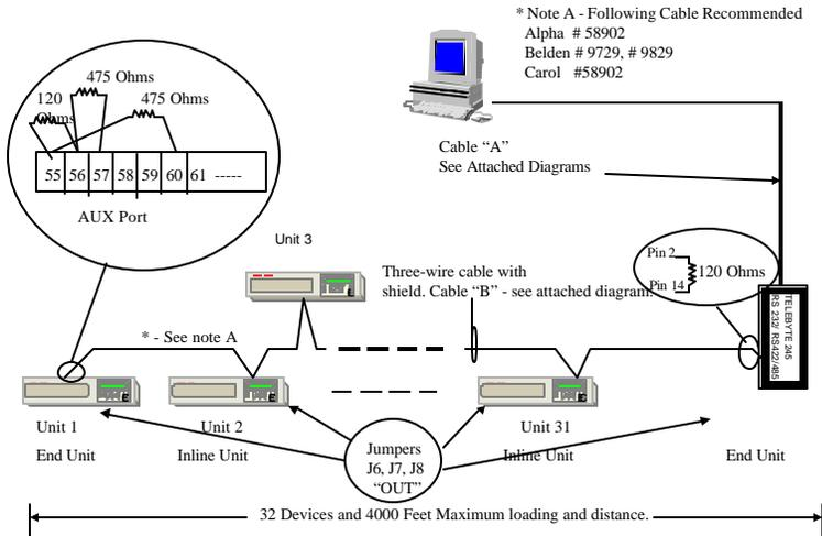
Figure 9 - Termination Using External Resistors On The IED's And Using The B & B Electronics Converter As An End Unit
