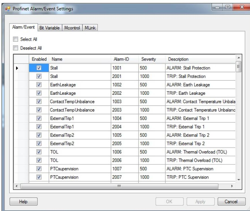
The *Name* and *Alarm-ID* are fixed and can not be changed. To enabled/disable an individual event, check/uncheck the checkbox under *Enable*. To change *Description* or *Severity* edit the cell with the new value.
