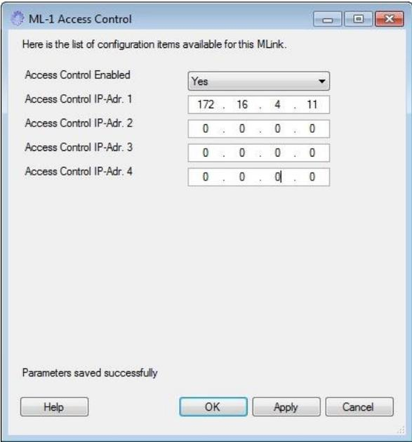
In above configuration only a PROFINET IO Controller with an IP address of 172.16.4.11 is able to establish communication with the *MLink*.
