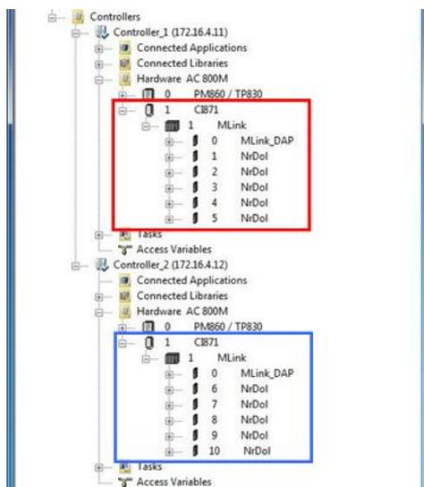
The red rectangle shows the first PROFINET IO Controller and the blue rectangle shows the second PROFINET IO Controller.
