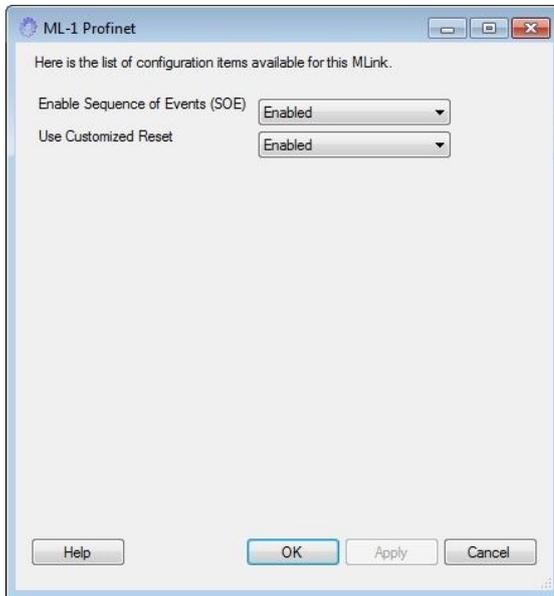
In addition it is also possible to enabled/disable individual events/alarms/trips. The message description that is sent to the IO Controller can be customized along with the severity of the event. As default severity 1 is used for events, 500 for alarms and 1000 for trips on a 1-1000 scale.
