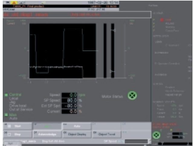
5 Close-up object display appearing in lower right-hand corner of the operator station monitor when the drive system is selected from any display. It shows actual values, interlocks, alarm statuses, etc.
