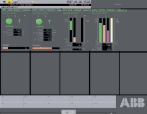
4 A group of objects can be combined to form a process group display, with each drive represented by setpoints and actual values. Interlocks, operating modes and annunciation of alarm, faults and events can be shown.
