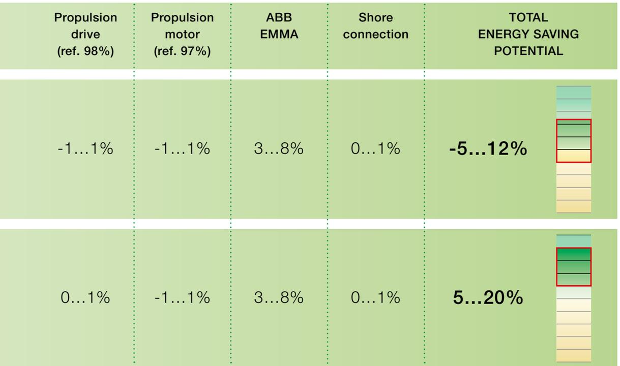
Savings within the 10,000 running hours when the voltage source inverter is selected instead of the traditional LCI-type (cruise ship standard as presented on page 65).
