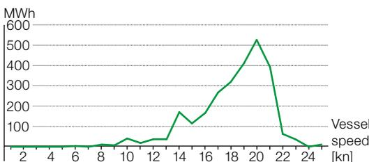
Savings within the 10,000 running hours when a synchronous motor is selected instead of an asynchronous motor. (cruise ship standard as presented on page 65).
