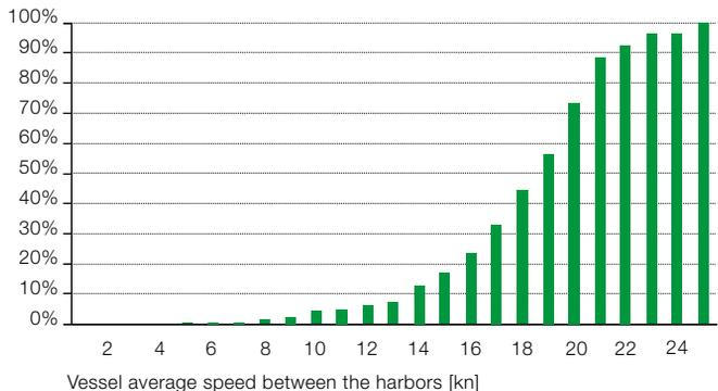
Share of cumulative energy consumption (% of the total consumption) of the 'Cruise vessel standard'. Calculations made for shaftline vessels in the customer project evaluation phase.
