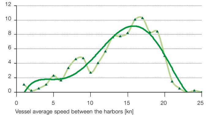
Cruise vessels operate according to the itinerary requirements, which are based on the season and area of operation. To determine a standard and comparable itinerary, cruises in the season 2009–2010 were analyzed. Based on approximately 1,000 legs from 150 cruises, ABB Marine established a cruise ship standard.
