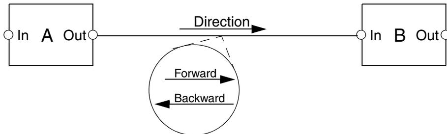
Figure 4. Point-to-point connection between two objects. The node names reflect the main direction of the signal. The blow-up shows in principle data flow.
