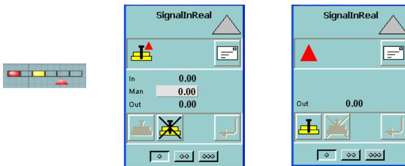
Figure 27. ParError indication on a Graphic Element Reduced Icon (left) and in Workplace faceplates (right).
