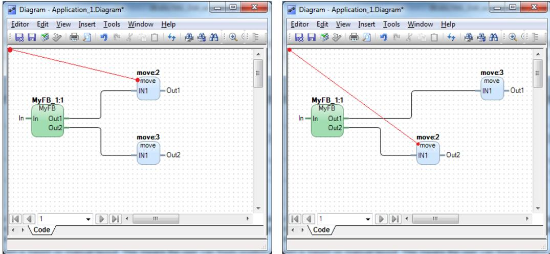
Figure 9. Flow Order Determined by Graphical Placement
