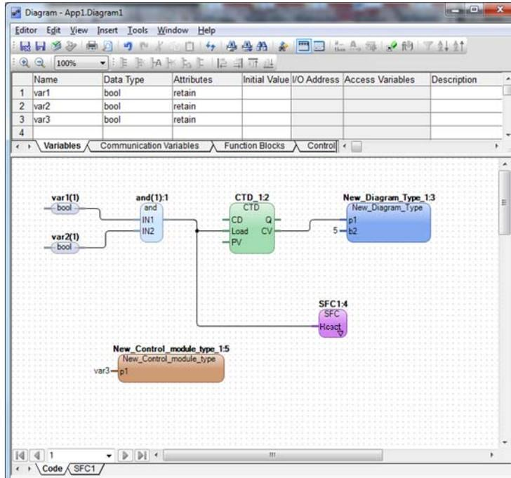
Figure 8. Diagram Example Containing Different Invocations
