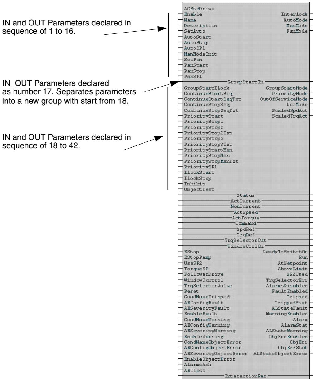
Figure 7. A graphical consequence for declared parameters.
