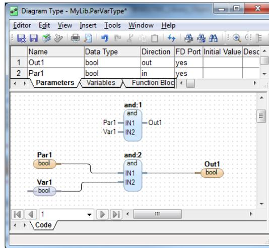
Figure 13. Connecting Parameters and Variables in Diagrams
