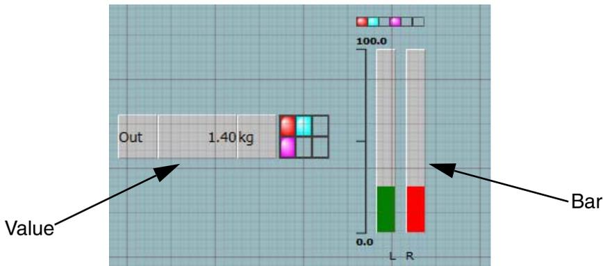
Figure 21. The additional display elements; (left) Value and (right) Bar.
