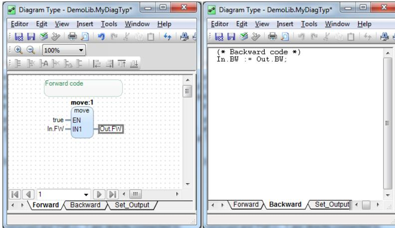
Figure 12. Diagram Type with Control Diagram (Forward) and Structured Text (Backward and Set\_Output) code blocks
