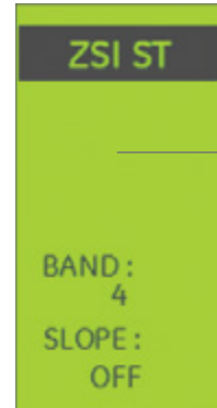
Trip Unit Toolkit Protection Settings Tab & LCD screen for configuring ST Restraint Settings
