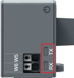
Fig. 5.18 Signals of Ekip Com Profibus DP -module
