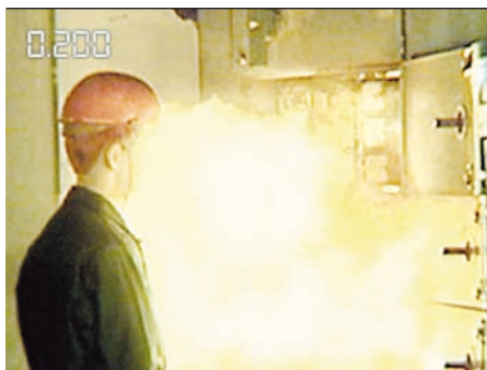
1a Arc accident without protection
