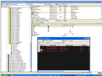
PLC Connect integrates individual signals in any connected controller, PLC or RTU with 800xA system. Operators receive process data in the same graphics regardless of the type of controller or communication protocol used.
