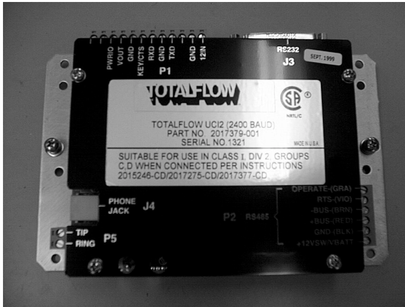
UCI2 (used to RS-232/485 conversion or dial-up modem operation)
