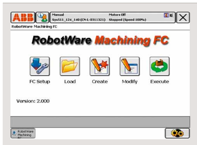
3 RWMFC graphic user interface on the Flex-Pendant of IRC5 controller
