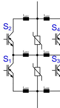
Fig. 11: only series arrester connection
