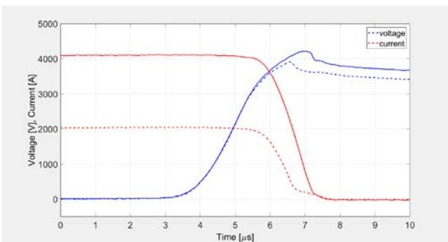
Fig. 8. Turn-off waveforms of a 4.5kV BIGT
