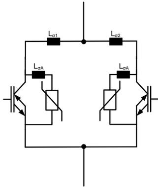
Fig. 9: parallel connection of two arresters
