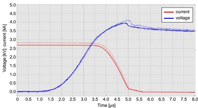
Fig. 10: turn-off waveform of two parallel connected IGBT with individual MO surge arrester in parallel
