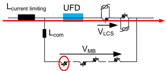
Fig. 1: Current flow during normal operation
