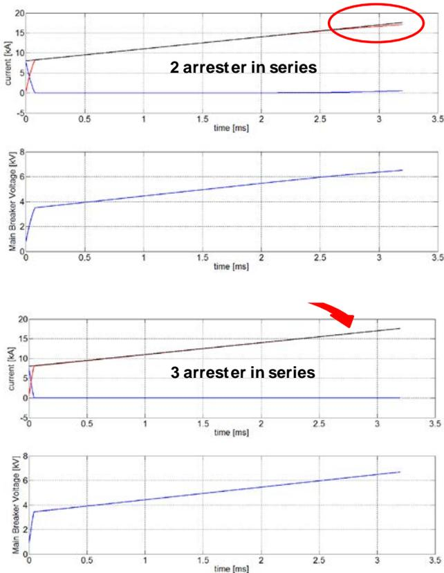
Fig. 5. Influence of number of arresters for “static” blocking. Top: 2 arresters in series / bottom: 3 arresters in series
