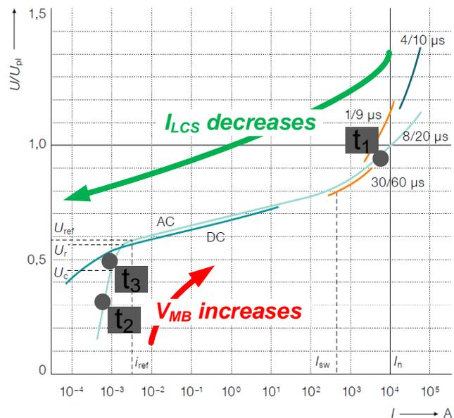
Fig. 4: Voltage vs. current characteristic of MO surge arrester
