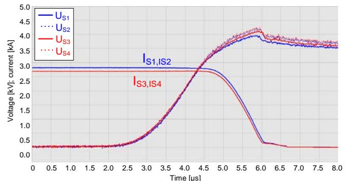
Fig. 13: turn-off waveforms of 4 semiconductors with paralleled surge arrester as in Fig. 12.
