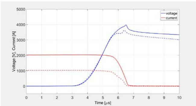
Fig. 7. Turn-off waveforms of a 4.5kV SPT+ IGBT
