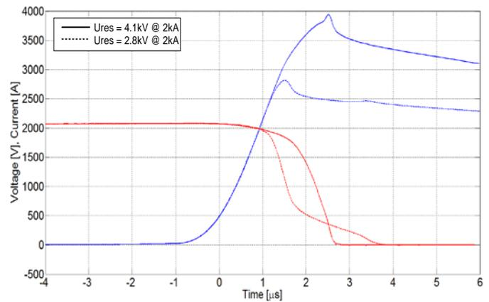
Fig. 6. Turn-off of a 4.5kV SPT+ IGBT with different arresters
