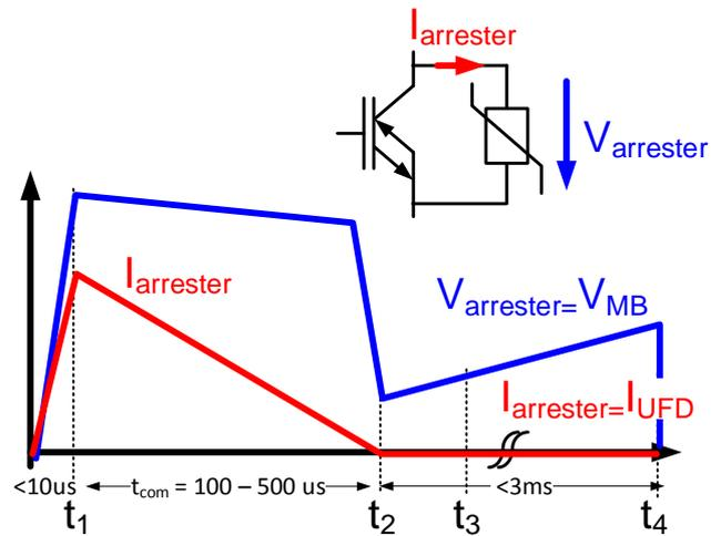
Fig. 3: Arrester voltage and current
