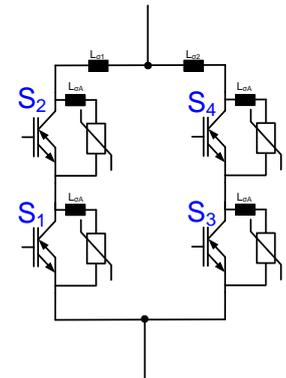
Fig. 12: series and parallel connection of arrester
