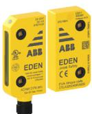
Eden is a non-contact safety sensor with the highest safety level for interlocking doors and hatches. Large mounting tolerances, M12 connectors and integrated reset speed up installation. Eden reduces cost by minimizing the number of cables and enables up to 30 sensors connected in series to reach the highest level of safety. IP69K, temperature tolerances of -40 to +70 degrees C and a minimum of surfaces edges makes it a perfect match for food and beverage applications.
