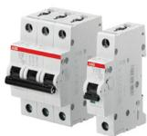
Miniature Circuit Breakers protect electrical installations against overloads and short-circuits, guaranteeing reliability and safety of operations. The System pro M compact S200 series are current limiting overcurrent protective devices. They have two different tripping mechanisms, the delayed thermal tripping mechanism for overload protection and the magnetic tripping mechanism for short-circuit protection.
