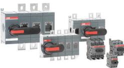
The OT range of switch disconnectors from 16 to 4000A is suitable for diverse applications such as machinery, power distribution and motor control centers. Thanks to a modular design, OT switches are available in different pole configurations. Mounting is possible in any direction and a wide offering of accessories is available.
