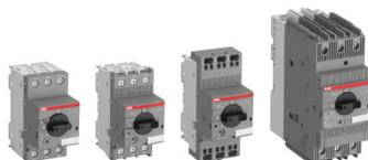
Manual motor starters are electromechanical protection devices for the main circuit. They are mainly used to switch motors ON/OFF manually and to provide fuseless protection against short-circuit, overload and phase failures. Fuseless protection saves costs, space and ensures a quick reaction under short-circuit condition by switching the motor off within milliseconds. Starter combinations are setup together with contactors and are available with screw or Push-in Spring terminals.
