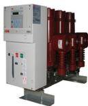
VD4/R are used in secondary MV distribution and in small transformer substations. They are available in fixed version with right-hand side operation mechanism. Circuit breakers with rated voltages up to 24kV can be fitted with current sensors and REJ603 self-supplied overcurrent release and can be used in unmanned substations without auxiliary power supply.
