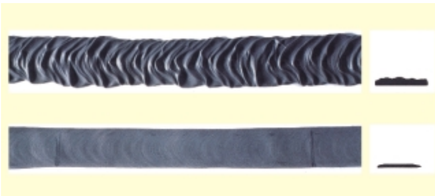
Weld sealing. The weld image exhibits a more uniform and flatter surface with robots than with manual sealing (top).
