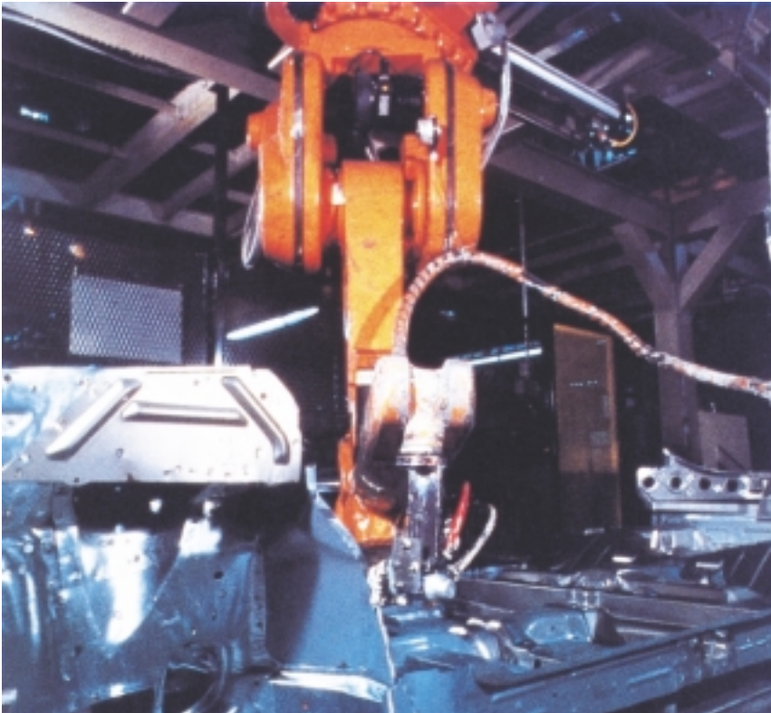
Robot sealing welds on the raw car body
