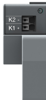
Fig. 5.7 Signals of auxiliary power supply module OXE1
