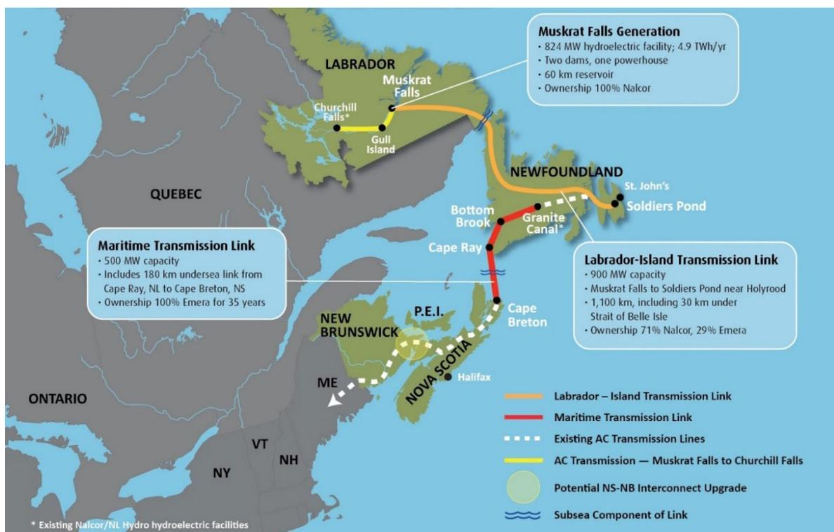
Figure 1 : Overview of Maritime Link and Labrador-Island Transmission Link.
