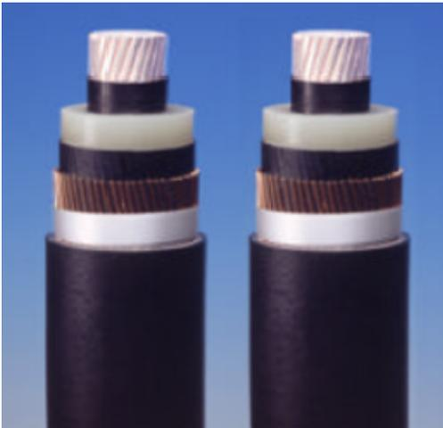
Fig. 4. Pair of extruded land DC cables showing from center outward: aluminum conductor, conducting XLPE-layer, dc-insulation XLPE, ground side conductive XLPE, copper shield wires, aluminum outer wrapping and outer sealing and mechanical protection..
