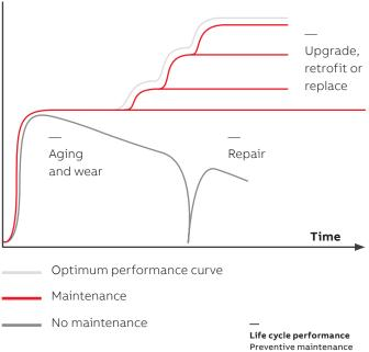
Preventive maintenance programs are designed to provide reliability and optimum performance, as represented by the horizontal red line.
