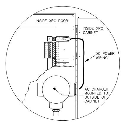
Figure 2-11 Mounting AC Charger
