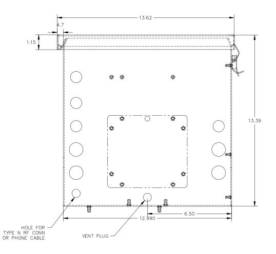
Figure 1-5 Bottom of Model XRC 6790
