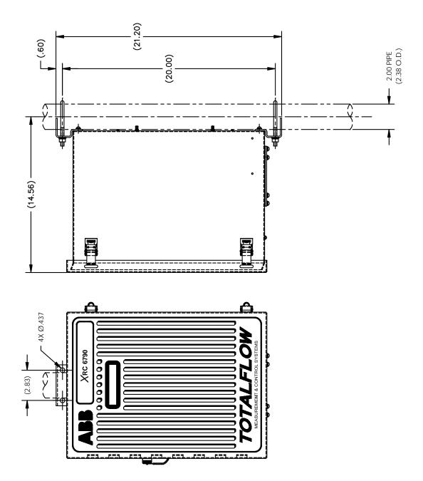
Figure 2-2 Model XRC 6790, Pipe Mounted
