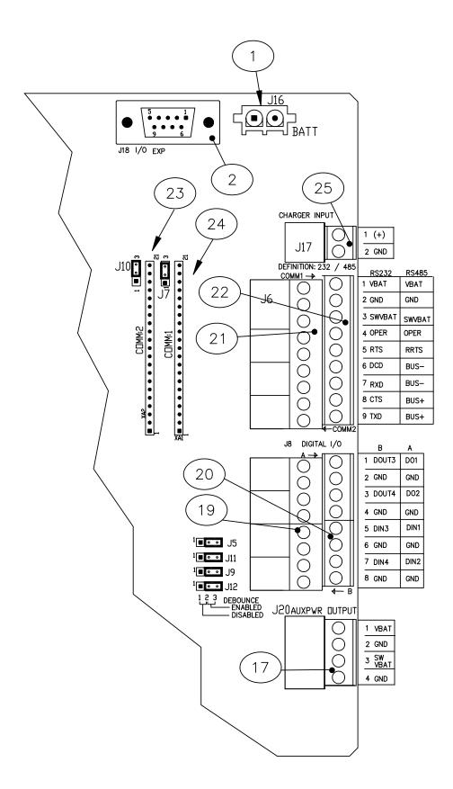
Figure 2-9 XRC-195 Board Cutout - Installation
