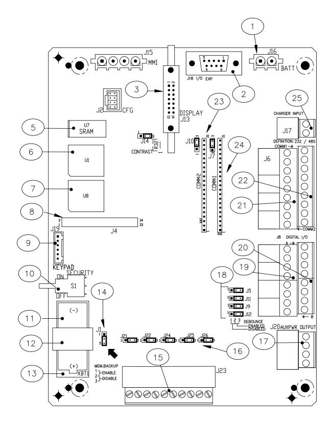
Figure 1-11 Complete View XRC-195 Board
