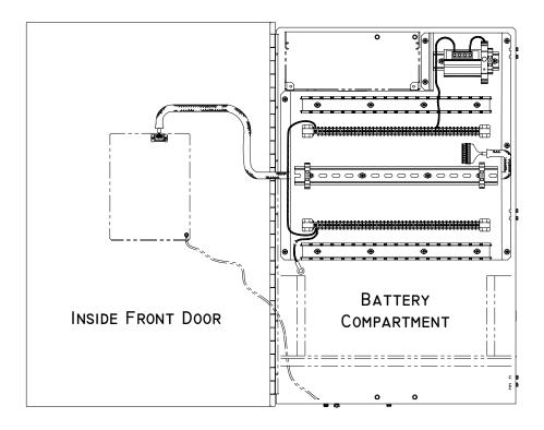
Figure 1-9 XRC 6890 Inside View with Busbar
