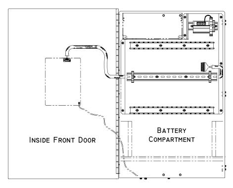
Figure 1-10 XRC 6890 Inside View without Busbar
