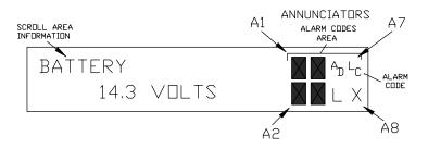
Figure 6-2 Liquid Crystal Display and Indicators
