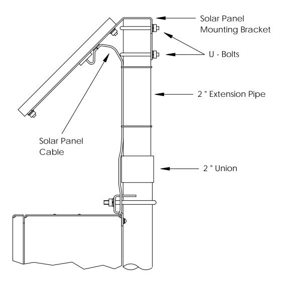
Figure 2-10 Typical Solar Panel Installation
