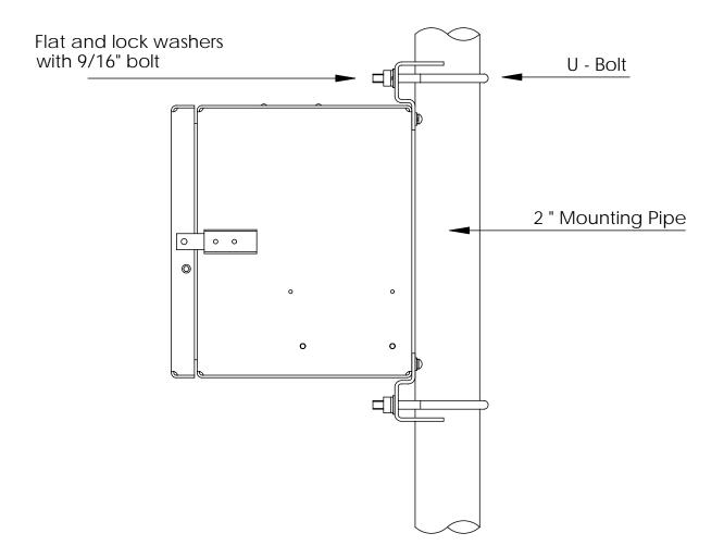
Figure 2-5 XRC Pipe Mounting
