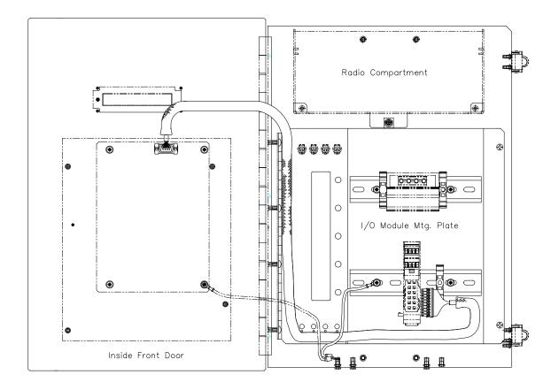
Figure 1-8 XRC 6790 Inside View with I/O Modules Installed
