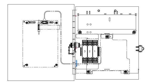
Figure 1-7 XRC 6490 Inside View with I/O Modules Installed
