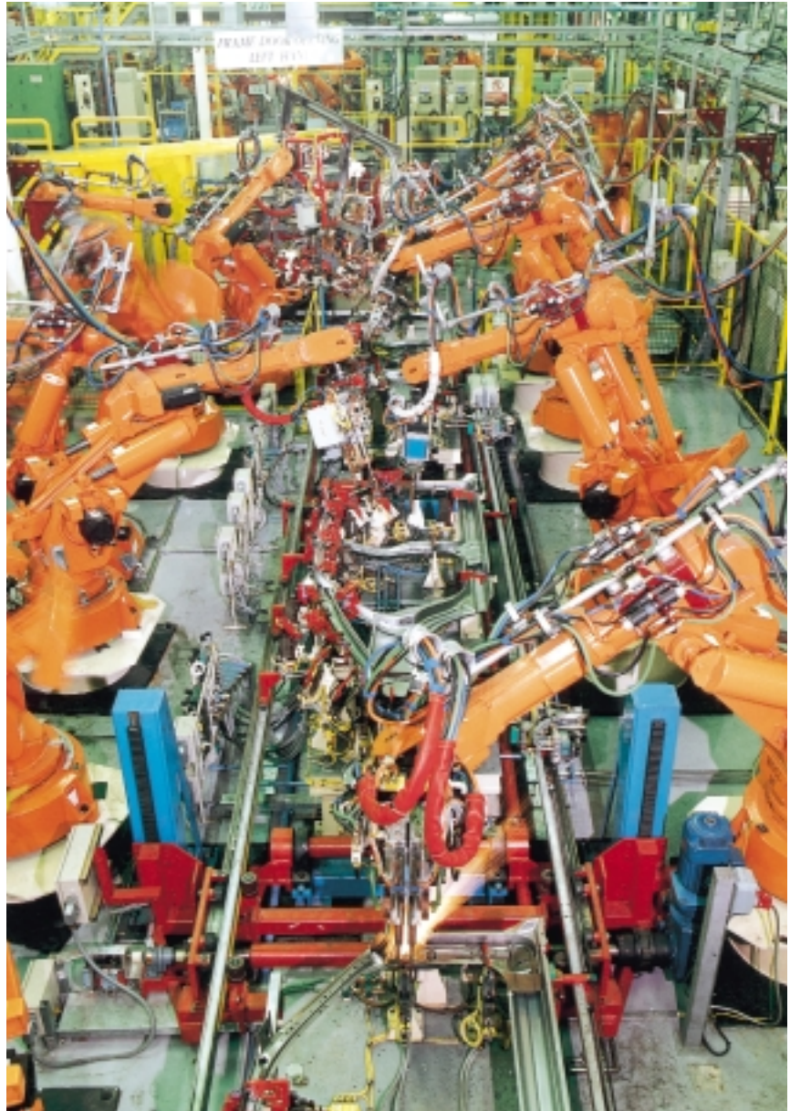
Welding body sides of the Vauxhall Vectra at Luton, UK
