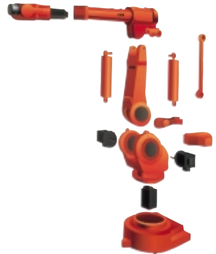
The modules of an IRB 6000 robot
