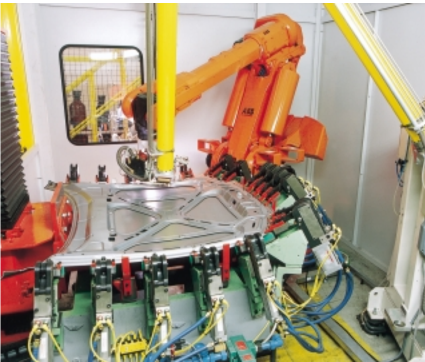
Final body respot line for the Vectra
