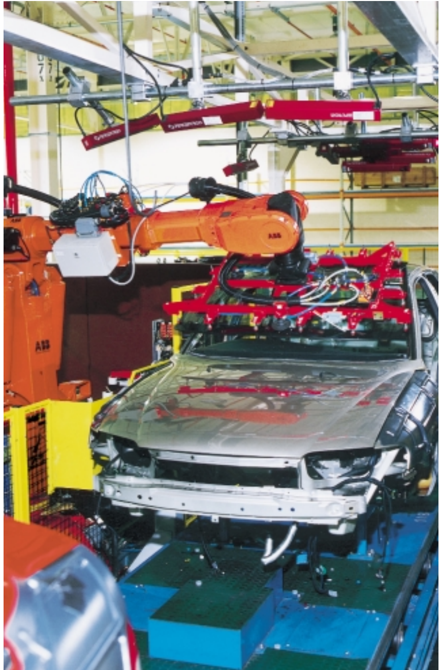
An ABB robot automatically inserts a front windscreen into the Vauxhall Vectra under the guidance of a vision sensing system.
