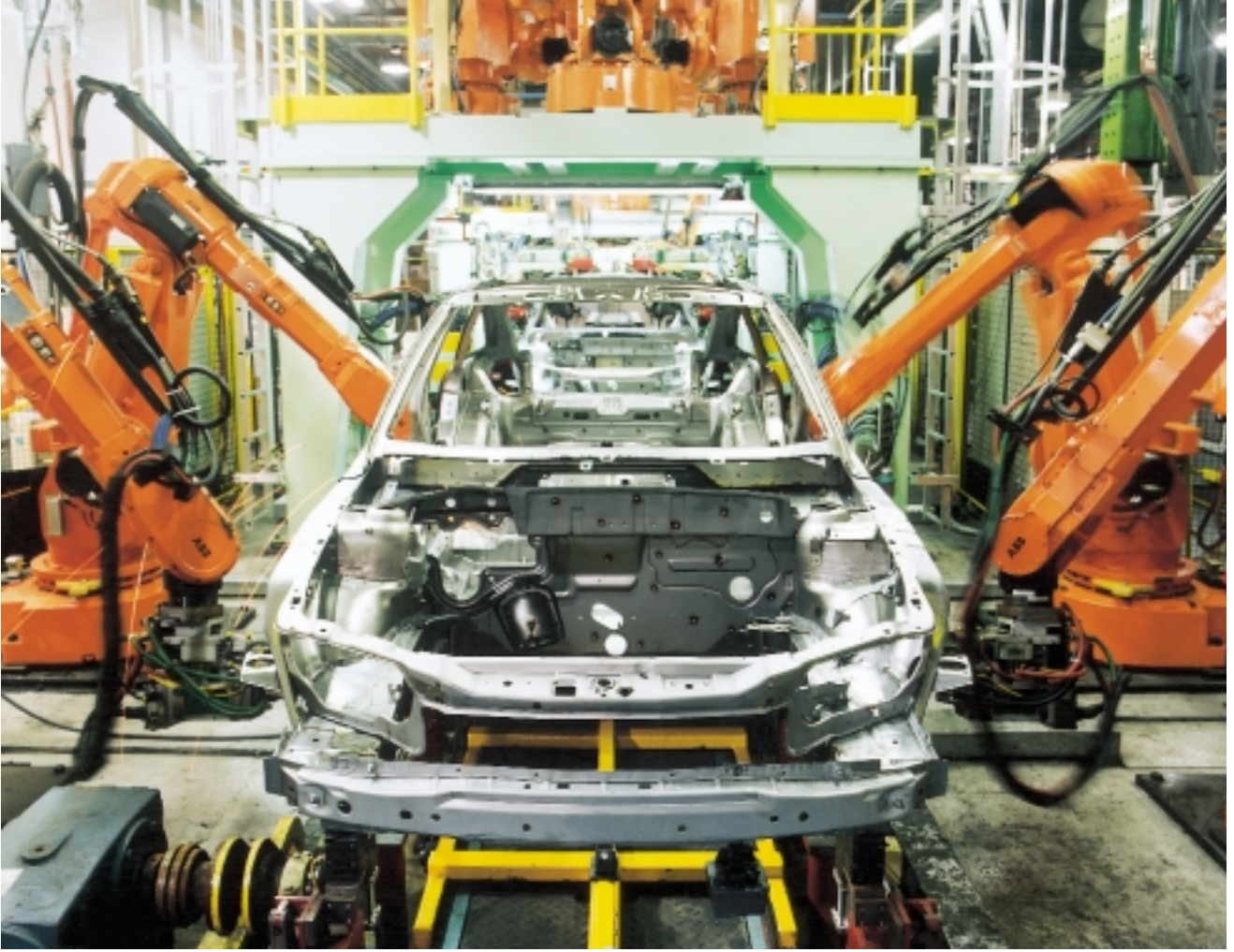
Final body respot line for the Vectra
