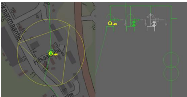
Figure 4. Remotely controlled CSS with fault indication in DMS system
