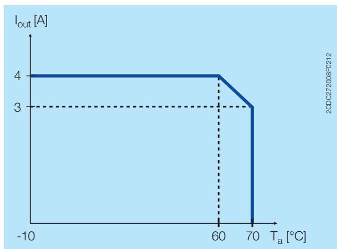
Characteristic curve of temperature at rated load
