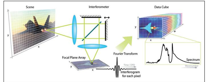
Schematized imaging Fourier transform spectroradiometer
