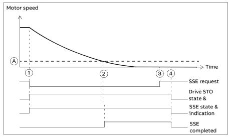
A Zero speed with encoder (parameter FSOGEN.52): Speed limit at which the motor has stopped, the safety function is completed and the SSE completed indication (parameter SSE.22) goes on. The acknowledgement becomes allowed.
