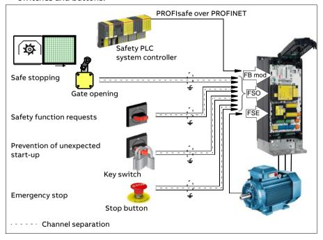
The FSO safety functions module is an option for the ACS880/DCS880 drives. The Safe torque off (STO) function is a standard feature on the ACS880/DCS880 drives.
