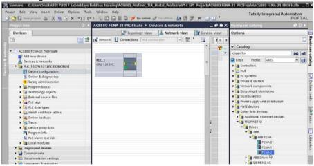
Open the FENA-21 device view and add (by dragging and dropping) the desired PPO and PS telegrams to slot 1 and 2. In this example, we use PPO7 and PS2 (Additional info in manuals).
