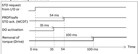
**Note:** The values shown above are applicable to ACS880 drives. The maximum response time for DCS880 drives is 550 ms.
