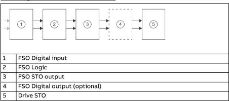
STO and other stopping functions with FSO include FSO subsystems Digital input, Logic, possible Digital output and STO output, and Drive STO. In the
