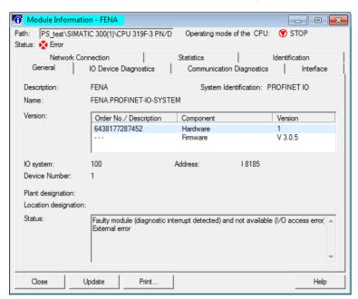
6. To check the Device number of the FENA module, select the General tab.
