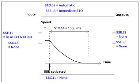
**Example 2 (with an encoder):** The figure below shows an example of the SSE function with immediate STO set-up when an encoder is used. Configure the
