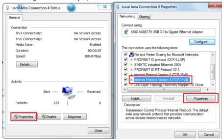
Finally, set your subnet to the same range as the PLC. Check that the IP address is not in use on the network.
