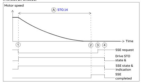
Time to zero speed (parameter STO.14): Time from the STO activation to the moment when the safety function is completed, the SSE completed indication (parameter SSE.22) goes on and the acknowledgement becomes allowed. You must set this to the estimated time in which the motor coasts to a stop from the maximum speed.
