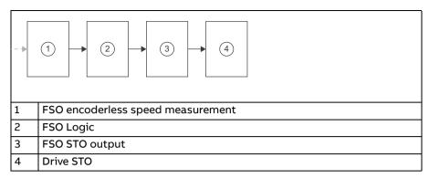
Safe maximum speed (SMS) includes the following subsystems: FSO encoderless speed measurement, FSO Logic, FSO STO output, and Drive STO.
