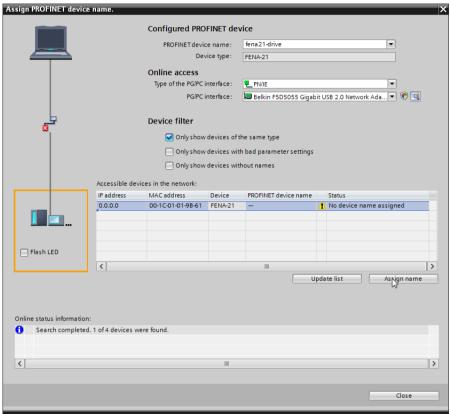
The PLC will assign a name and IP address to the selected FENA and drive parameter group 51 values will update accordingly.
