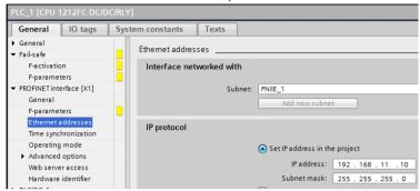
11. In **Advanced options**, set PLC minimum cycle time for I/O and PROFINET communication (PROFINET cycle time).
