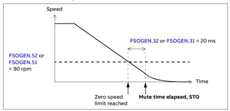
**Example 2**: Zero speed limit is reached with the SS1 function (or SSE with emergency ramp), a negative SBC delay (parameter SBC.12 STO SBC delay) is configured in the STO function:
