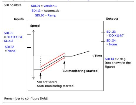
The SDI functions use SAR1 parameters to monitor and/or define the deceleration ramp (SDI with ramp monitoring). See section Configuring SAR on page 354.
