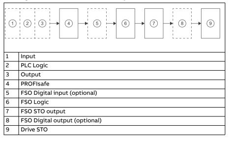
PROFIsafe can replace digital inputs and/or digital outputs of the FSO. For example, it is possible to use PROFIsafe input and FSO output in the same configuration.
