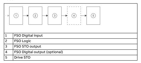
Prevention of unexpected start-up (POUS) includes the following subsystems: FSO Digital input, FSO Logic, FSO STO output, FSO Digital output (optional), and Drive STO.
