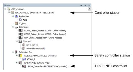
Right-click on the PROFINET controller CM579-PNIO-Master and add the FENA module to the PROFINET IO network.
