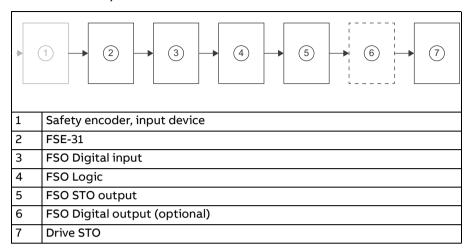
Safely-limited speed (SLS) with encoder includes the following subsystems: safety encoder (not provided by ABB), FSE-31, FSO Digital input, FSO Logic, FSO STO output, FSO Digital output (optional), and Drive STO. Block diagram is equal to SDI and SS1-r.
