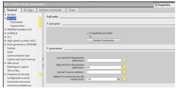
In the F-parameters submenu, define the maximum allowed safety program execution interval. If this value is exceeded, PROFIsafe goes to safe state (watchdog).
