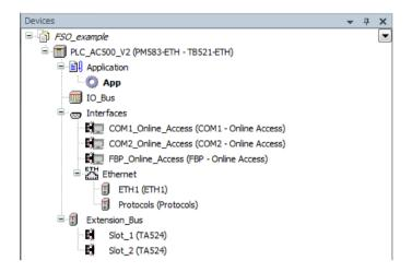
Next, add the necessary controller devices to the PLC project. First add the safety controller to slot 1 (make sure that the physical controller is in the same slot). Right-click on the slot, select Add object, and pick the SM560-S safety controller from the list.
