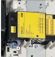
5. Connect the supplied four-wire cable to FSO terminal X111. Connect the other end of the cable to the drive STO connection (XSTO connector). ABB recommends that you use the cable delivered with the FSO module. For the specifications for a customer-defined cable, refer to section STO cable and data cable between FSO module and drive on page 514.
