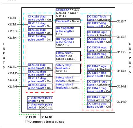
Note: The safety relay inputs and outputs must be configured so that in the Safe state the circuit is disconnected (0 V).
