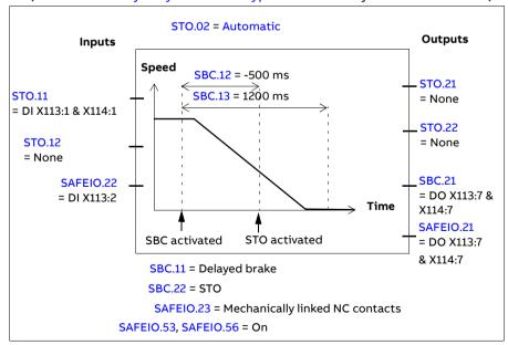
**Example 2 (with an encoder):** The figure below shows an example of the SBC before the STO set-up when an encoder is used. Configure the safety encoder
