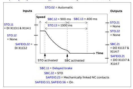
**Example 2 (with an encoder):** The figure below shows an example of the SBC after the STO function set-up when an encoder is used. Configure the safety encoder interface first (see section Configuring the safety encoder interface on page 309).
