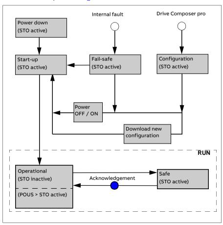
At power-up, the FSO goes into the Start-up mode. During the power-up process. FSO is in Safe state (STO active). It performs start-up checks and. according to the configuration, enters the Operational state either automatically or after an acknowledgement request from the FSO I/O or from a safety PLC.
