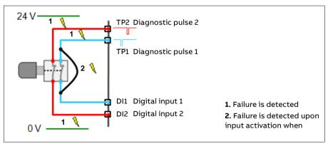
**Note:** If only one of the redundant inputs is activated upon a safety function request, the FSO module activates the safety function in which the input is configured but it cannot be acknowledged before the failure is repaired. To acknowledge the safety function, you must set both input channels down and up at the same time or, switch the power off and on.
