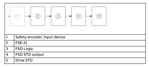
Safe maximum speed (SMS) includes the following subsystems: safety encoder (not provided by ABB), FSE-31, FSO Logic, FSO STO output, and Drive STO.
