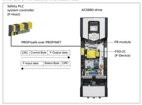
The FSO-21 safety functions module and the FB module are installed on the ACS880 drive. The safety PLC is connected to the FB module, which communicates with the FSO module. The safety PLC activates safety functions via the PROFIsafe communication bus. The user can also activate safety functions from an I/O device (for example, an emergency stop button) which is connected to the FSO module.
