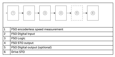
Safely-limited speed (SLS) without encoder includes the following subsystems: FSO encoderless speed measurement, FSO Digital input, FSO Logic, FSO STO output, FSO digital output (optional), and Drive STO. Block diagram is equal to SS1-r function
