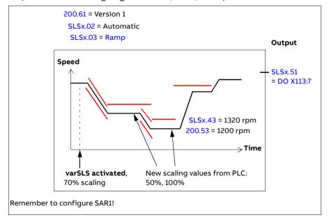
See also section SLS reaction when modulation is lost during deceleration ramp, with ramp monitoring on page 148.
