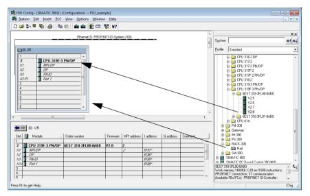
5. When you install the controller station to the rail, select Industrial Ethernet as the subnet for the controller station.
