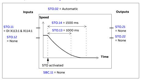
**Example 2 (with an encoder):** The figure below shows an example of a simple STO function set-up when an encoder is used. Configure the safety encoder
