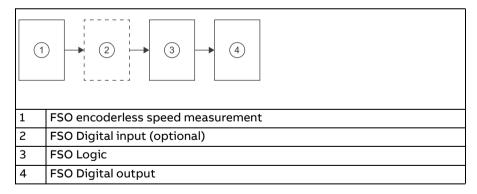
Encoderless SSM includes the following subsystems: FSO encoderless speed measurement, FSO Digital input (optional), FSO Logic, and FSO Digital output.
