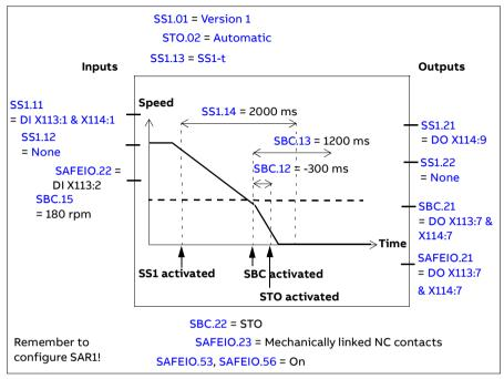
Note: This figure shows the case when an encoder is not used.
