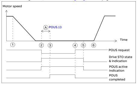
A POUS delay for completion (parameter POUS.13): Sets a delay for POUS completed indication. The POUS completed indication (parameter POUS.22) goes on after this delay.
