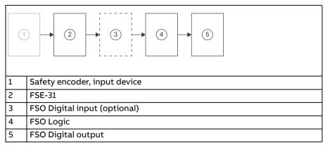
Safe speed monitor (SSM) with encoder includes the following subsystems: safety encoder (not provided by ABB), FSE-31, FSO Digital input (optional), FSO Logic, and FSO Digital output.
