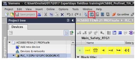
25. Scan for accessible devices (start search). Note that a firewall can block
