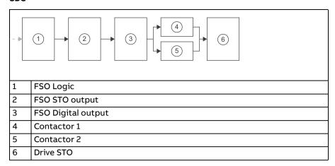
Safe brake control (SBC) includes the following subsystems: FSO Logic, FSO STO output, FSO Digital output, Contactor 1 and 2 (can be provided by ABB), and Drive STO.
