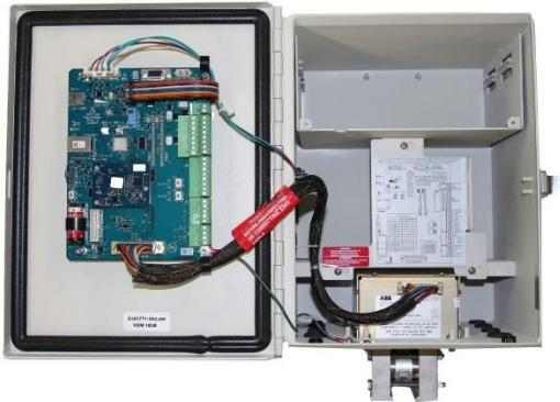
Figure 1-2: XRC<sup>G5</sup> inside the enclosure
