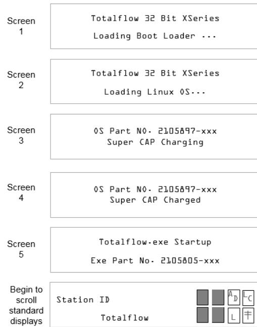
**IMPORTANT NOTE:** If the LCD fails to display the startup sequence, try adjusting the contrast first as described in section [10.6 Adjust the LCD contrast](#). If adjusting the contrast does not show any items on the LCD, see section [12 Troubleshooting](#).
