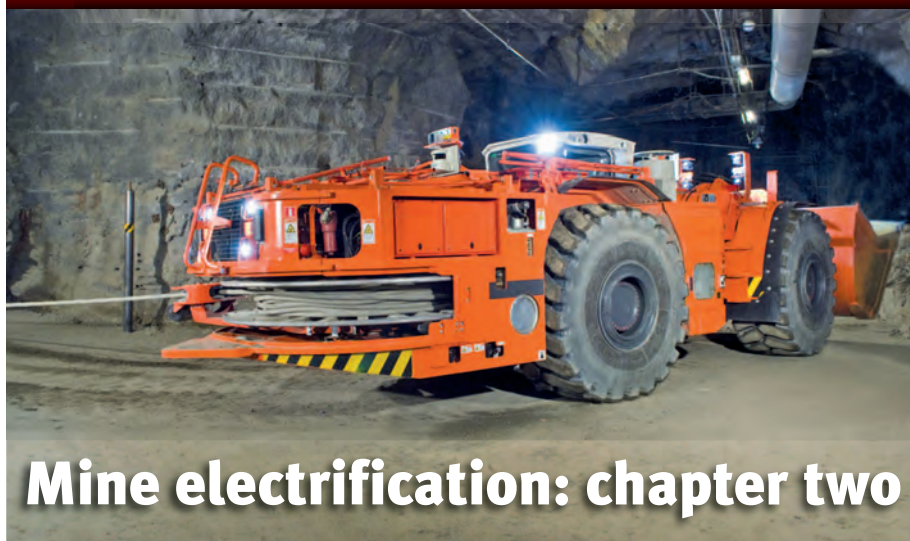
The Sandvik LH514BE is understood to be a combination of tethered cable and battery – battery for tramming and cable operation for mucking
