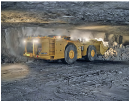
The 15 t R1700XE will be Cat's first battery-powered underground loader
