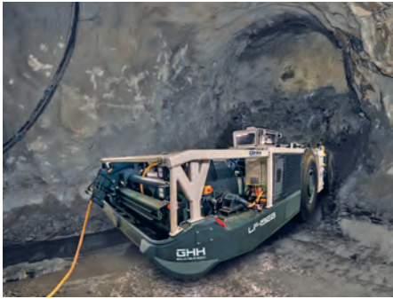
GHH's new tethered battery-electric loader, the LF-19EB, is predominantly for soft-rock applications and specifically designed for loading into a feeder breaker
