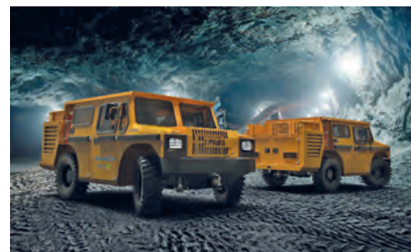
The Paus MinCa 5.1 E can handle inclined ramps up to 45°
