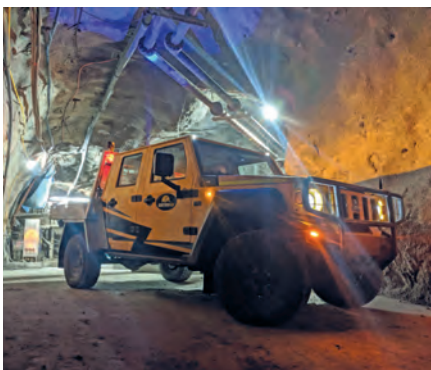
The Bortana EV uses the chassis of a diesel-powered Agrale Marruá, with 3ME Technology supplying the system integration expertise and component supply, and Safescape providing the design and engineering expertise
