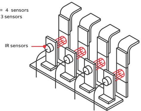
**Module power contact temperature monitoring**
