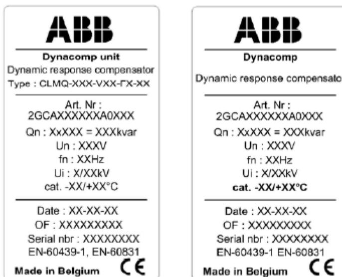
Figure 3: DYNACOMP identification tags for each individual cubicle (left) and for the complete DYNACOMP (right)图3:左边为每个 DYNACOMP 单元的识别标签右边为 DYNACOMP 整体单元识别标签
