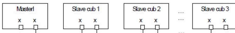
**Note:** The RVT-D located in the Master cubicle is always at the end of the CAN control bus. It should be noticed that the other end of the CAN control bus should be loaded by an “end of line load resistor”. This is done by setting ON the dip switch Nr6 noted “CAN” of the last Dynacontrol board 提示：安装在主单元上的 RVT-D 作为 CAN 控制总线终端。尤其要注意，若 CAN 控制为最后一个工作站点，则需连接一个终端电阻。其做法可通过 Nr6 的拨码开关进行设置。
