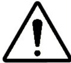
**WARNING: Conductive dust may cause damage to this equipment. Ensure that the DYNACOMP is installed in a room where no conductive dust is present.** 警告：确保 DYNACOMP 安装在没有导电粉尘的室内，以避免导电粉破坏该设备。
