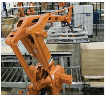
Assembling the perfect flat pack: Svedplan, Sweden Svedplan, part of the Licentia Group, is a fast emerging producer of flat pack furniture that has deployed a team of nine ABB robots, four for de-palletizing and five for packing, to improve competitiveness and reduce risk to manual handlers.
