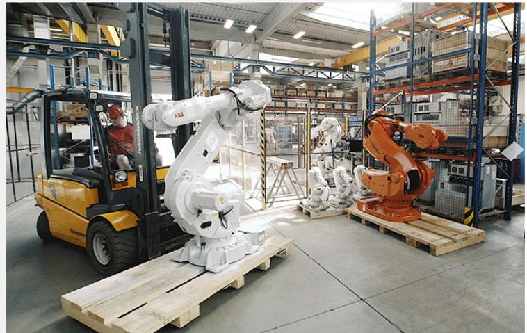
Over the last 25 years, ABB’s remanufactured robot teams have given new life to thousands of robots. These previously owned robots, along with peripheral equipment such as controllers and manipulators, are refurbished to “like-new” conditions at one of ABB’s Global Remanufacture & Workshop Repair Centers.
