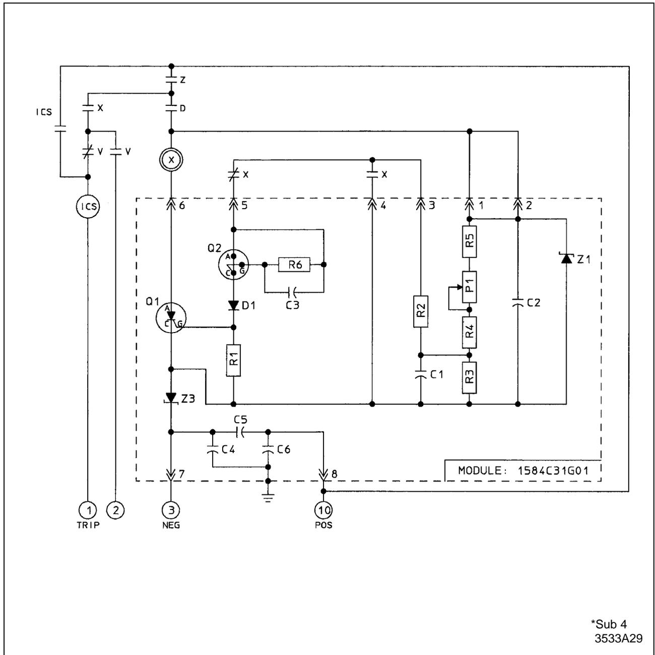
Figure 14. Relay Type KLF-1, Time Delay Schematic for Class 1E Application
