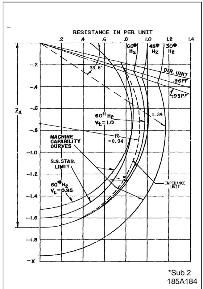
Figure 8. Typical Machine Capability Curves and Sample KLF-1 Settings - Per Unit Impedance
