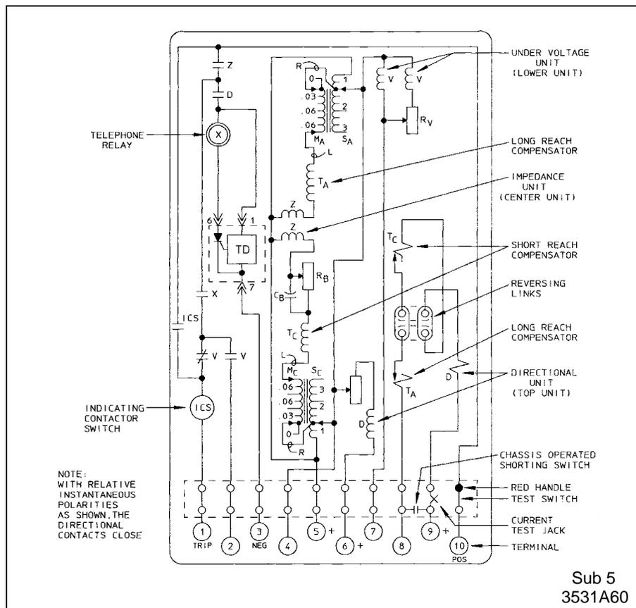
Figure 3. Internal Schematic of Type KLF-1 Relay in FT41 Case
