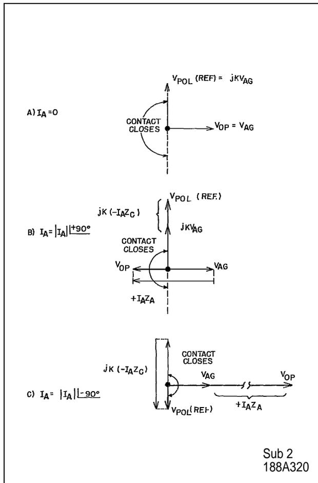
Figure 6. Effect of Compensator Voltage ( $Z_C$  is positive)
