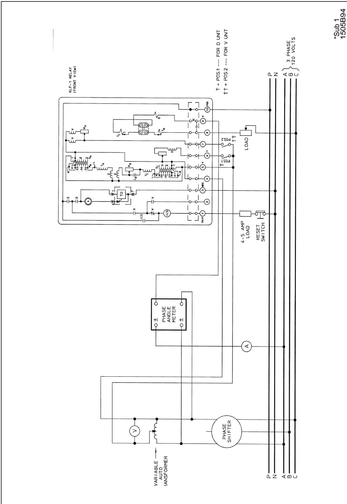
Figure 9. Diagram of Test Connections for KLF-1 Relay
