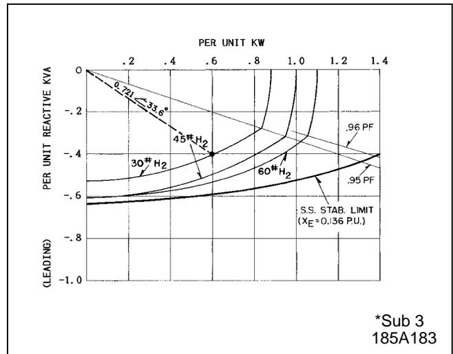
Figure 7. Typical Machine Capacity Curves Plotted on a Per Unit Basis (183,500 kVA, 45# H2, 18 KV, 0.9 pf, 0.64 SCR, inner-cooled, 3600 rpm)
