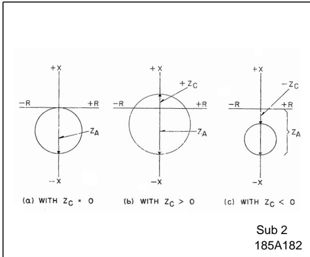
Figure 5. R-X Diagram Characteristics with Various  $Z_C$  Compensator Settings
