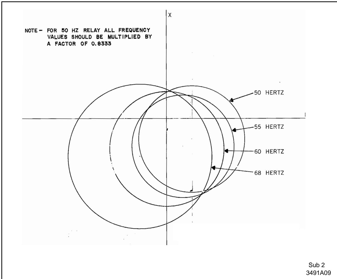
Figure 13. KLF-1 Frequency Response For Impedance Unit For 60 Hz Relay
