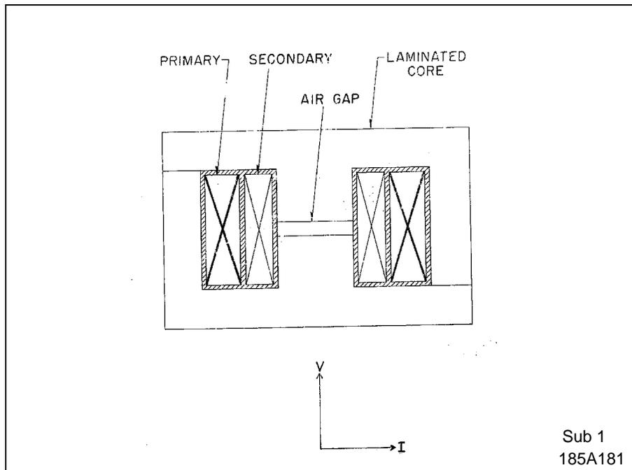
Figure 2. Compensator Construction
