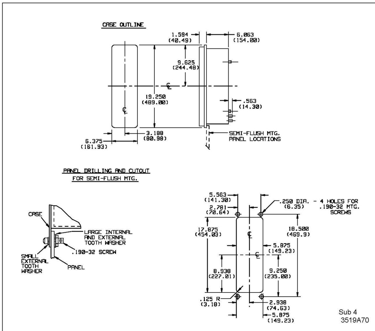
Figure 15. Outline and Drilling Plan for the Type KLF-1 Relay in the FT-41 Case (Class 1E)
