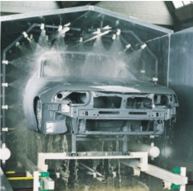
RoDip spray degreasing in the full-scale prototype installation. This process ensures optimum cleaning of the outside body surface.
