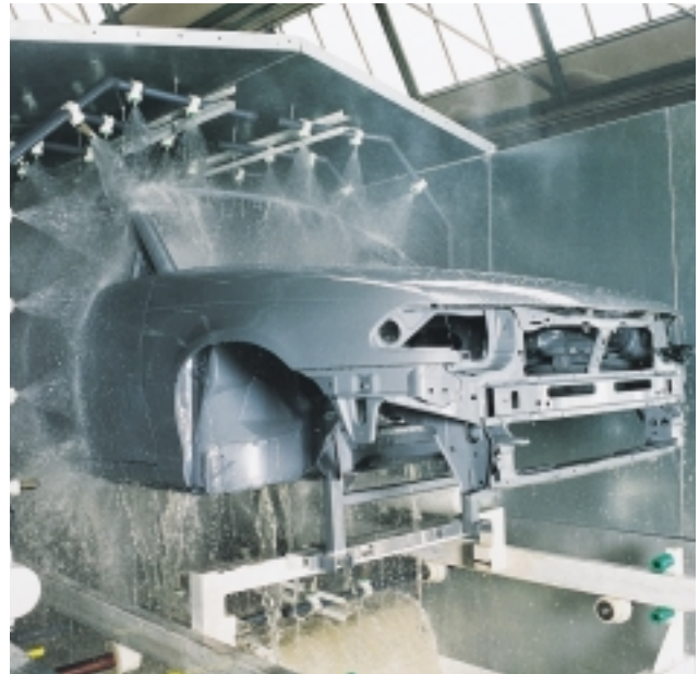
RoDip spray degreasing in the full-scale prototype installation. This process ensures optimum cleaning of the outside body surface.
