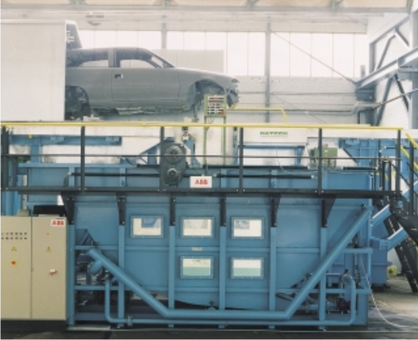
Pilot installation for car body pretreatment with the ABB RoDip system. The car bodies are dipped in the tanks by rotating them 180°
