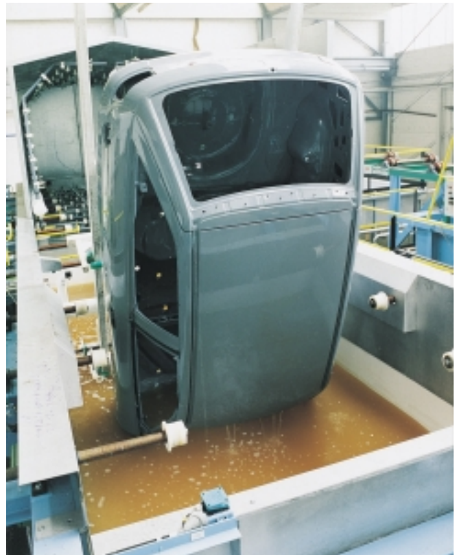
Car body being tilted during RoDip degreasing in the prototype installation. The purpose of this process is to ensure optimum cleaning
