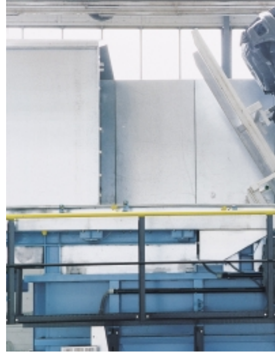
Pilot installation for car body pretreatment with the ABB RoDip system. The car bodies are dipped in the tanks by rotating them 180°
