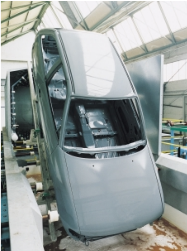
Car body being tilted during RoDip degreasing in the prototype installation. The purpose of this process is to ensure optimum cleaning
