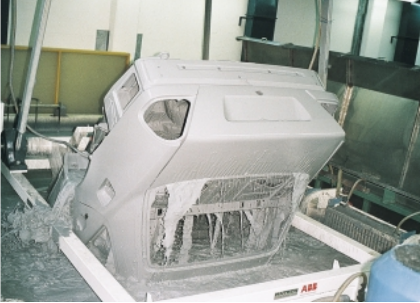
Removing a car body from the tank in a RoDip electrocoating installation
