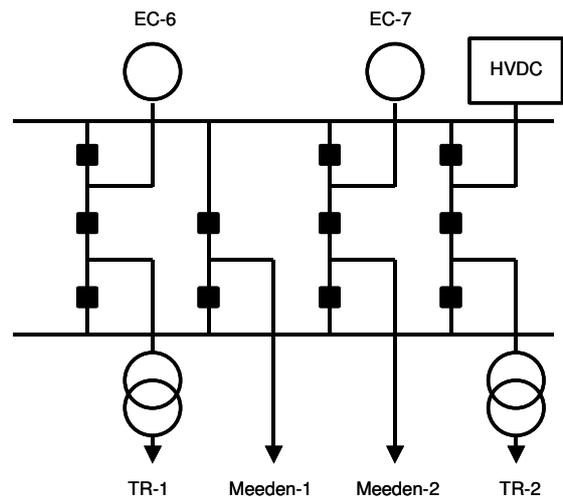
Figure 6 Schematic diagram substation Eemshaven
