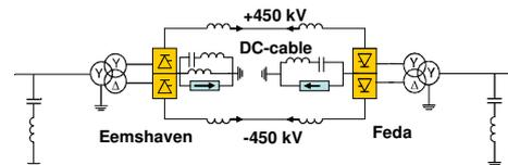
Figure 1. NorNed main circuit configuration
