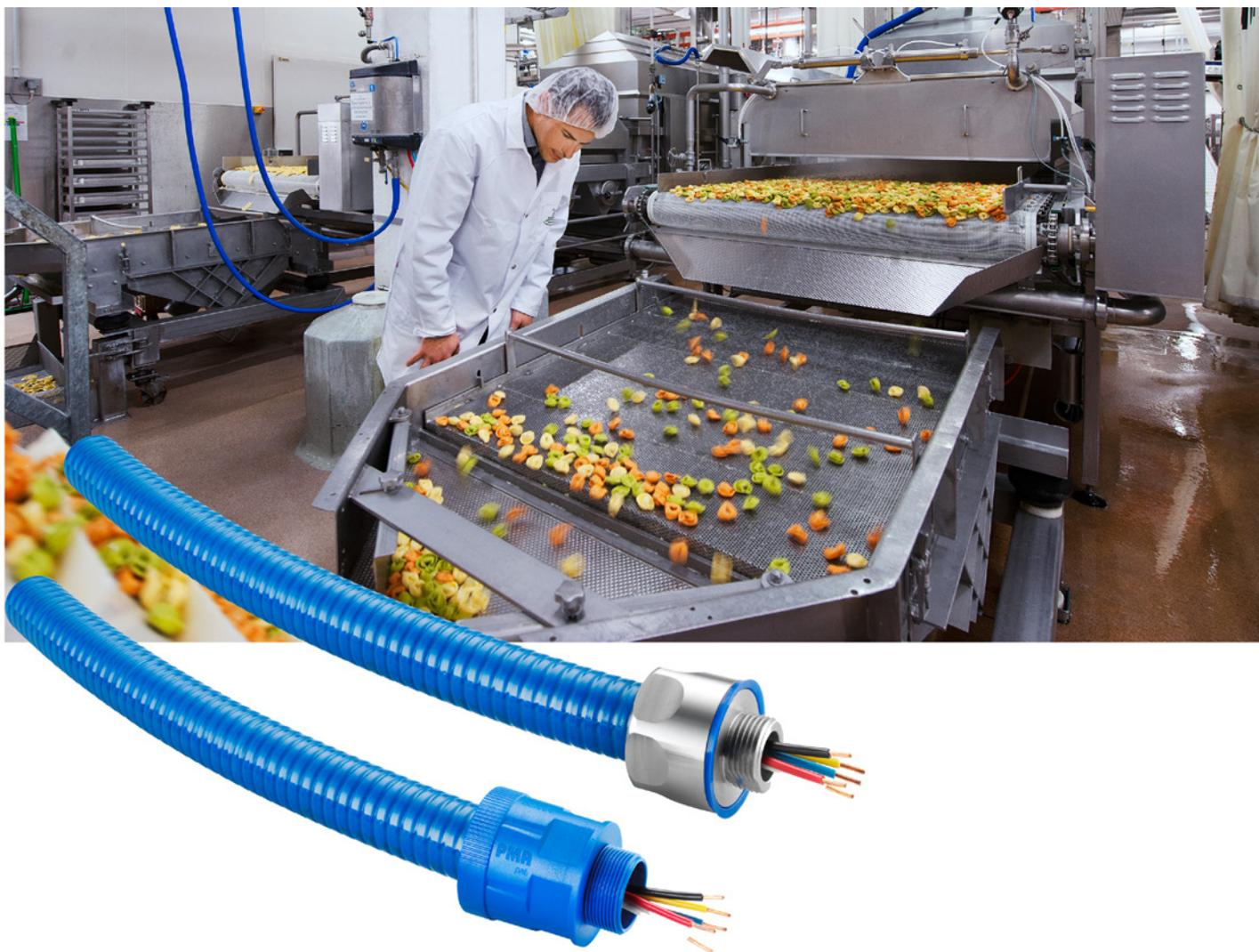
— The IP69-rated PMA cable protection range for the food and beverage industry offers a choice of two high-specification fittings. The JKNH nylon fitting is made from FDA-compliant material and offers both excellent chemical resistance and tool-free quick installation. The JENQ single-piece fitting is made from 316L stainless steel and is ideal for applications that have to meet stringent hygiene standards.
