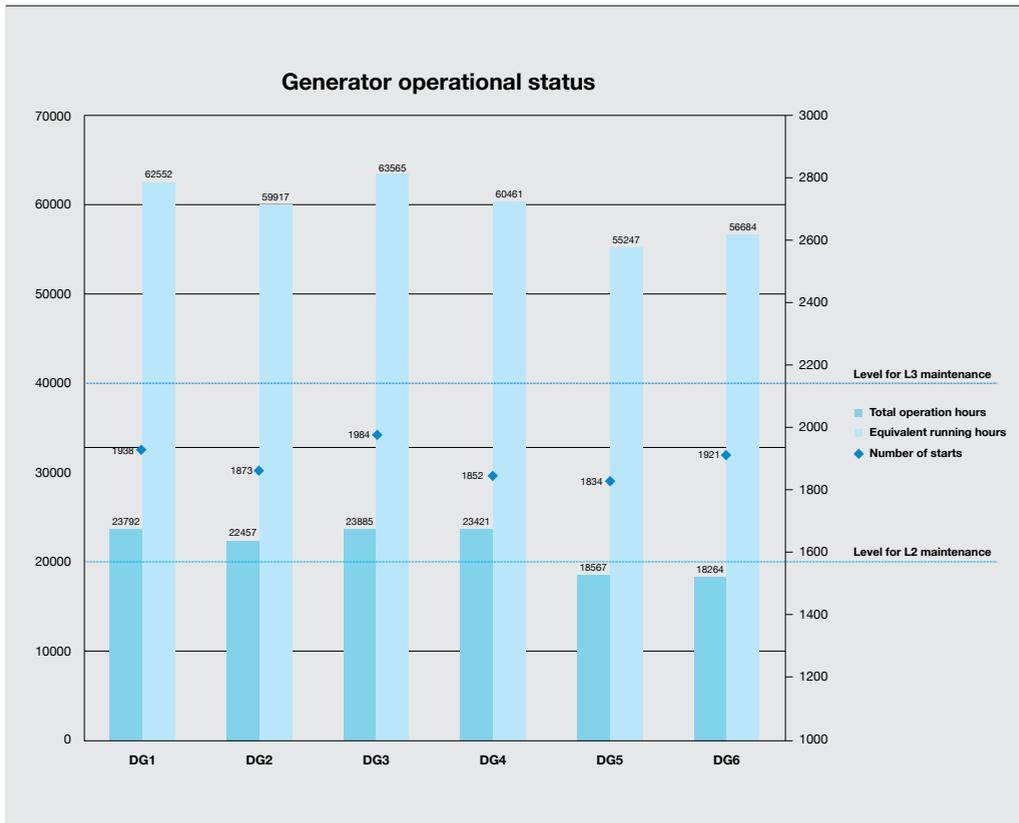
It is also possible to extend the maintenance interval by proper planning of power management and engine configuration. Also, when the vessel changes operational profile, it should be a common approach to reevaluate maintenance needs and not just follow a calendar-based maintenance plan.
