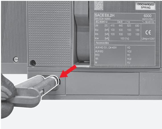
**4** By means of the cross screwdriver unscrew the 4 screws fixing the front cover to the circuit breaker main structure.
