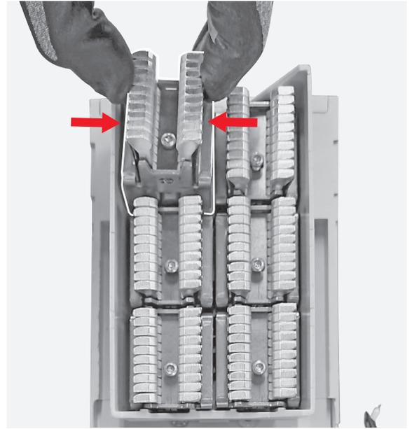
**221** Manually remove the spacers located below the claw contacts.
