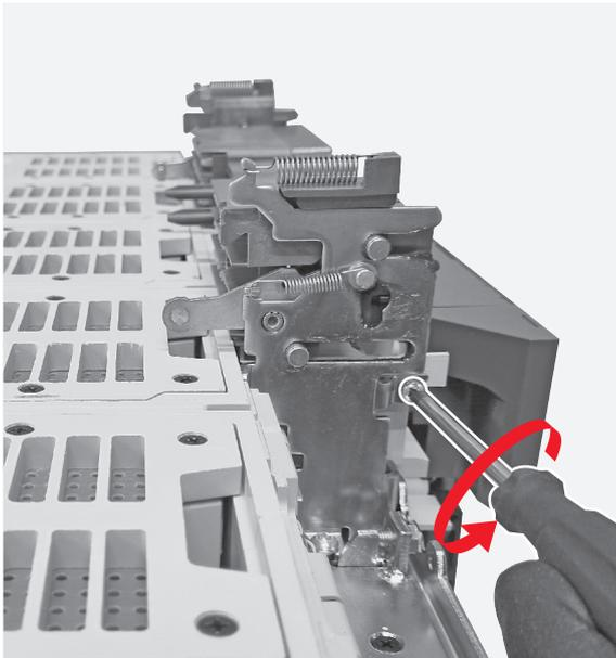
**21** By means of the cross screwdriver unscrew the 1 + 1 screws fixing the 2 sides walls located at both sides of the sliding contacts block to the circuit breaker main structure.
