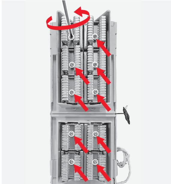
**220** Push the claw contacts as indicated by the arrows and after manually remove the claw contacts.
