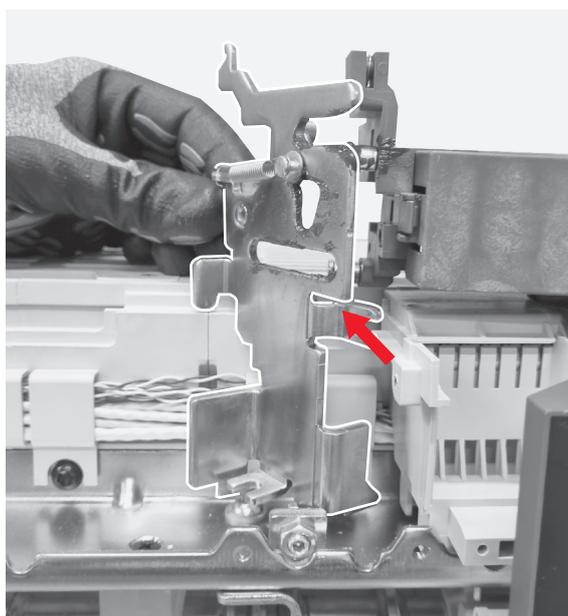
**23** Move the sliding contacts block as shown in the picture and by means of the torx key unscrew the 6 screws fixing the base and the cover.
