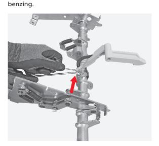
**210** Manually remove the lever.
