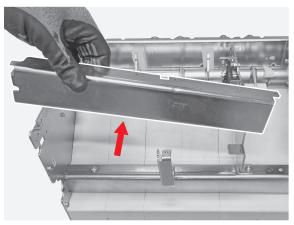
By means of the cross screwdriver unscrew the 2 screws fixing the right support to the circuit breaker main structure.
