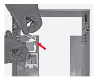
**9** Manually remove the T.U. Reset assembly.
