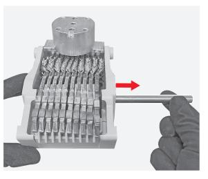
**253** Manually unhook both appendixes of the insulation protection.
