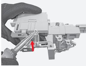
By means of the pliers unhook and remove the spring indicated by the arrow mounted on the MID main structure.
