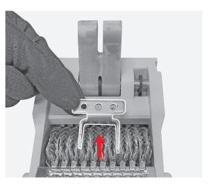
Manually remove the fixed contact.
