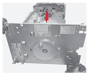
By means of the cutter start removing the 3 labels located on the left shoulder and manually complete the operation.
