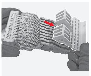
Manually remove the 10 springs mounted on the contacts holder.
