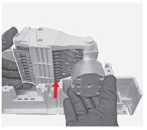
Manually remove the jumper.
