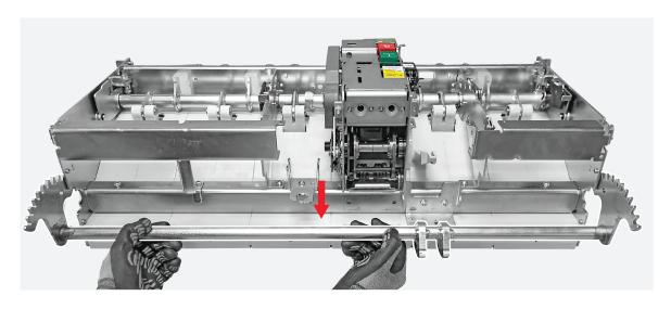
By means of the torx key unscrew the 3 screws fixing the motor fixing plate and the support mounted in the bottom part of the circuit breaker main structure and after manually remove the motor fixing plate and the support.
