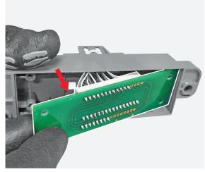
Manually pull and remove the wiring cables set.
