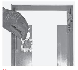
By means of the flat screwdriver push the pin as indicated by the arrow and after let the the spring and the T.U. Reset signalling plug automatically separate from the T.U. Reset metal support.
