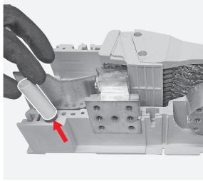
Manually remove the insulating protection.
