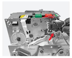
By means of the flat screwdriver remove the 2 benzings fixing the 2 levers to the operating mechanism.
