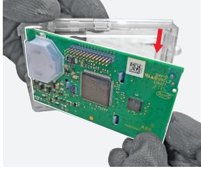
**67**By means of the flat screwdriver remove the "i TEST" pushbutton from the HMI LCD cover.
