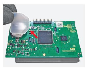
Manually remove the display support.
