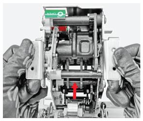
**200** manually remove the operating mechanism.
