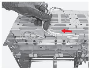
By means of the flat screwdriver remove the 3 clips.
