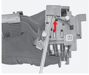
By means of the flat screwdriver unhook the right side wall from the sliding contacts main assembly as indicated in the picture.
