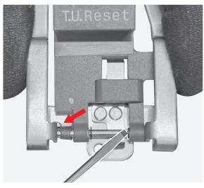
By means of the torx key remove the 2 screws fixing the plug to the circuit breaker front cover.
