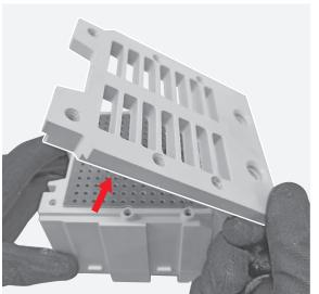
**233**By gravity let the 2 filters and the spacer separate from the arching chamber shell.
