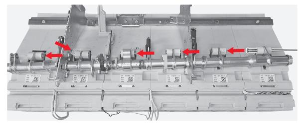
**204**Manually remove the operating shaft assembly.
