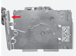
**166** Manually remove the assembly shaft.
