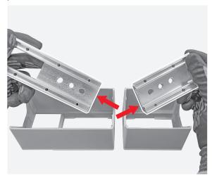
Disassembly operations illustrated at pictures 219,  $\dots$ , 224 must be performed on the other 5 poles.
