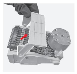
Manually remove the pin.
