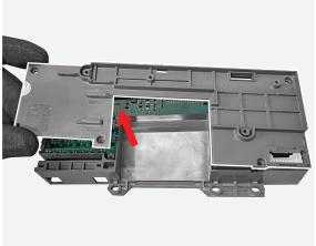
By means of the flat screwdriver unhook the trip unit printed circuit board.
