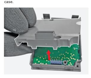
Manually remove the Ekip measuring blind
