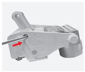
Manually remove the pin and the tie rod.
