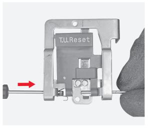
**8**By means of thr torx key unscrew the 2 screws fixing the T.U. Reset assembly to the front cover.
