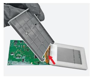
Manually separate the gasket from the display.
