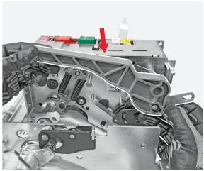
By means of the flat screwdriver remove the benzing and let the pin and the lever separate by gravity.
