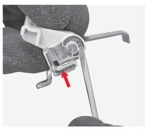
By means of the flat screwdriver push the pin as indicated by the arrow and let the the I/O shaft, the I/O shaft group support and the leaf spring constituting the I/O shaft group separate.
