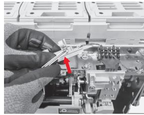
By means of the flat screwdriver remove the 2 clips and after manually complete the removal.
