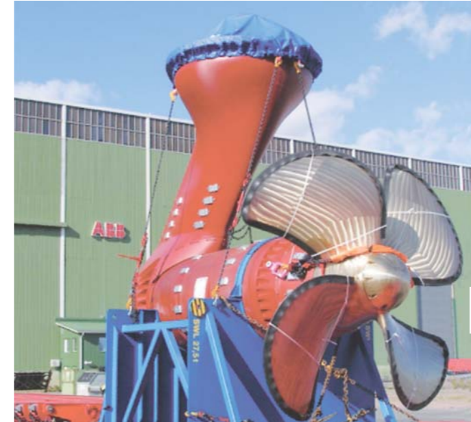
Azipod® CO propulsor ready for shipment from ABB factory
