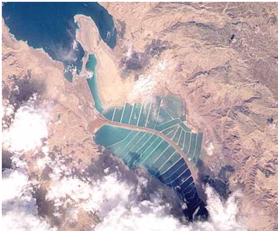
Satellite image of the southern basin of the Dead Sea, with the APC salt ponds on the right and the Israeli salt ponds on the left, separated by a central canal that is also the international border between the two countries. The Dead Sea is one of the saltiest bodies of water in the world, with a salinity level of 33.7 percent, about ten times that of the average sea or ocean. Source: NASA.
